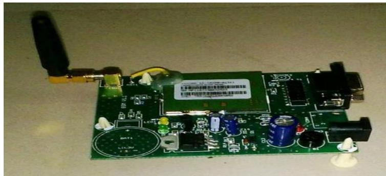
**Figure 5- GSM Modem**
