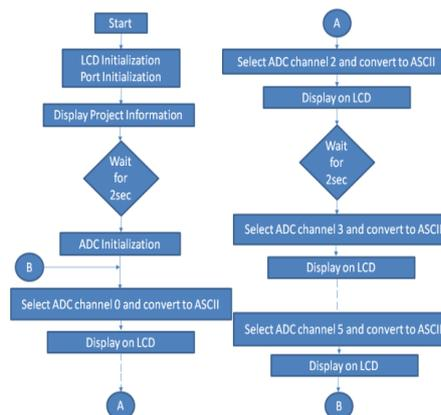
Figure 8-Process flow during start and monitoring
