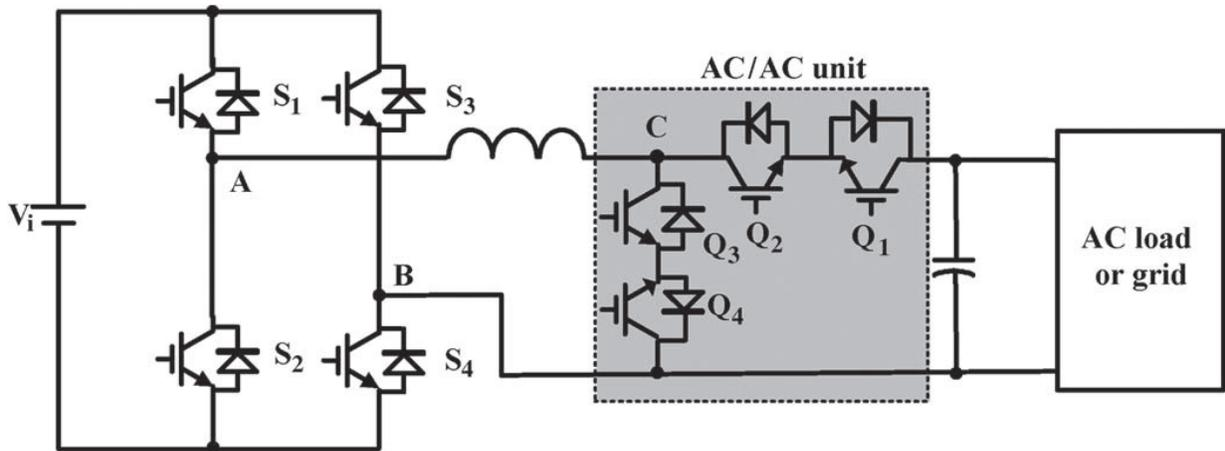
Fig.4. Proposed active buck boost inverter
