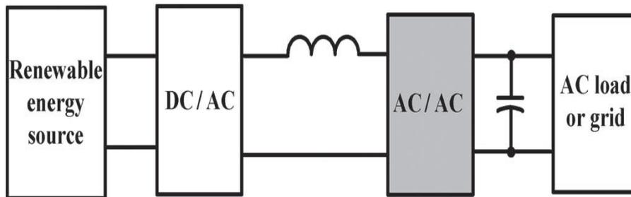
Fig.2. Structure of Active buck boost inverters
