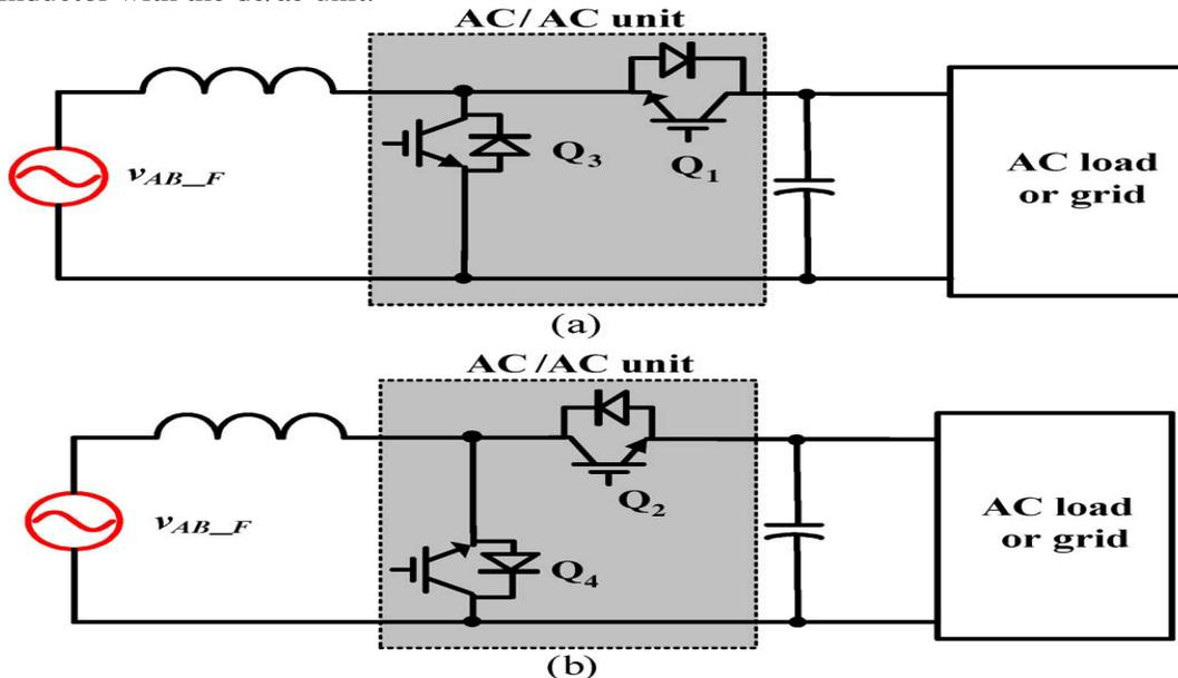
Fig.5. Proposed active buck boost operation mode
