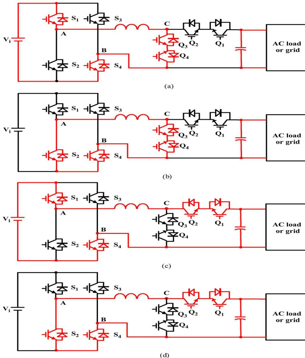
Fig.6. Proposed active buck boost operation mode of operation
