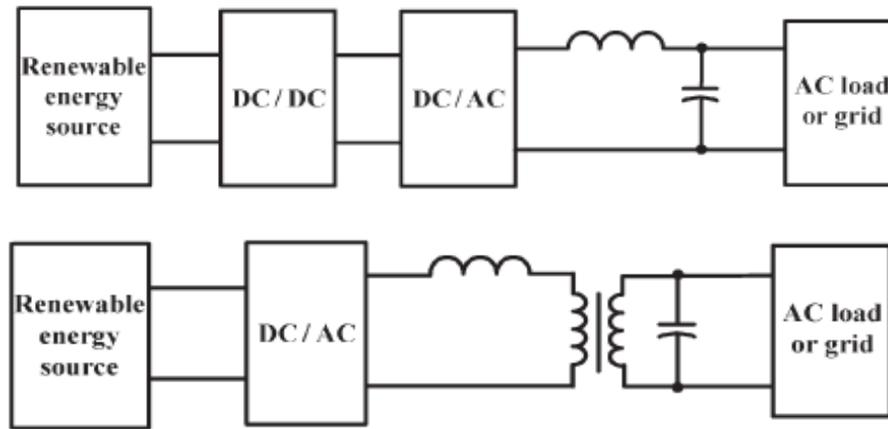
*Fig.1. Existing buck boost inverter schemes*
