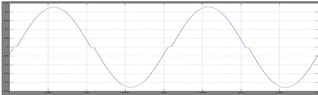
Fig 12. Output current in boost mode
