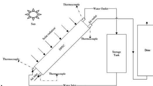
**Fig. 9: Hybrid Solar Drier and Water Heater System**
