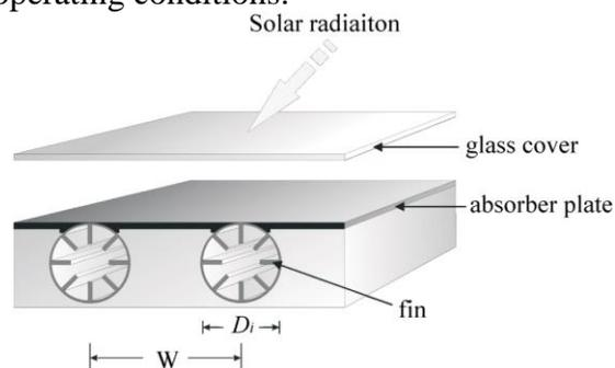
*Fig. 3: Sheet-and-tube solar water heater with internal fins*
