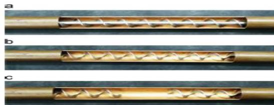
*Fig. 4: Helical tape is inserted in the tube.*
