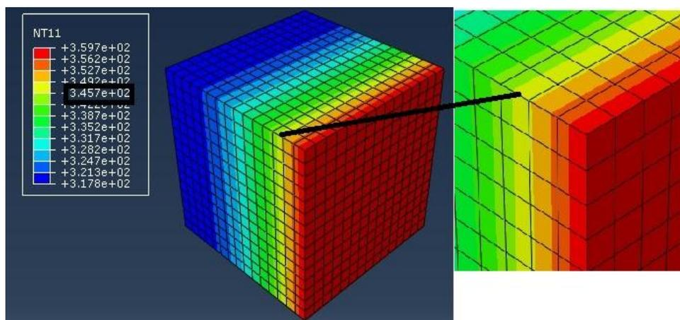
Figure 3. Temperature distribution in concrete
