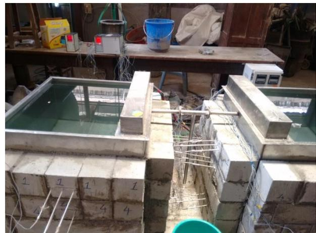
Figure 2. Steel lined concrete water tank
