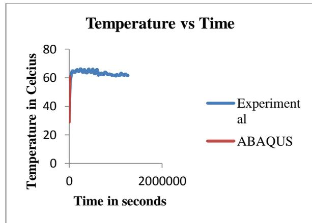
*Figure 5. Variation of temperature with time (Depth 80mm)*
