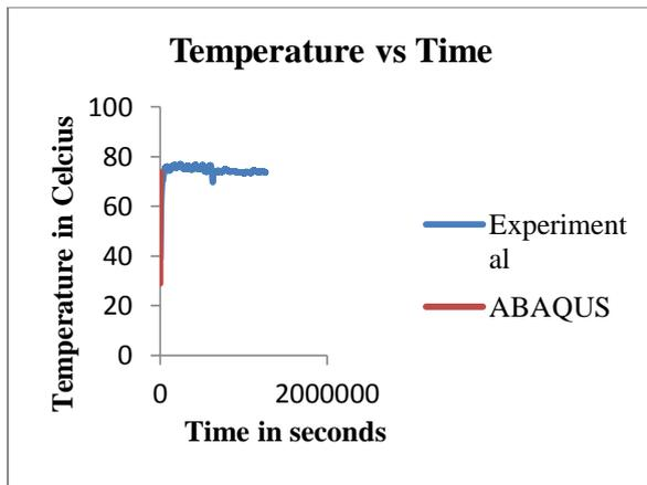
*Figure 4. Variation of temperature with time (Depth 135mm)*
