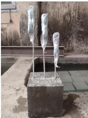
Figure 1. Concrete block with RTD sensors
