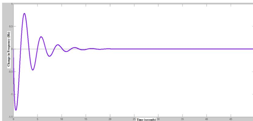
*Fig 7 frequency response of conventional PID controller*
