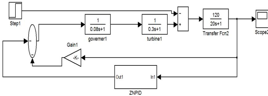
**Fig 8 MATLAB Diagram of PID Controller for single Area Load Frequency Control**
