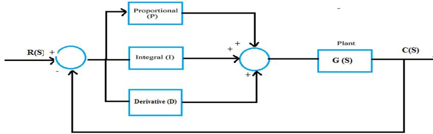
Fig 3 PID Controller
