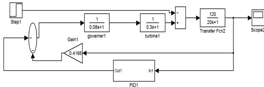
*Fig 6 MATLAB Diagram of PID Controller for single Area Load Frequency Control*
