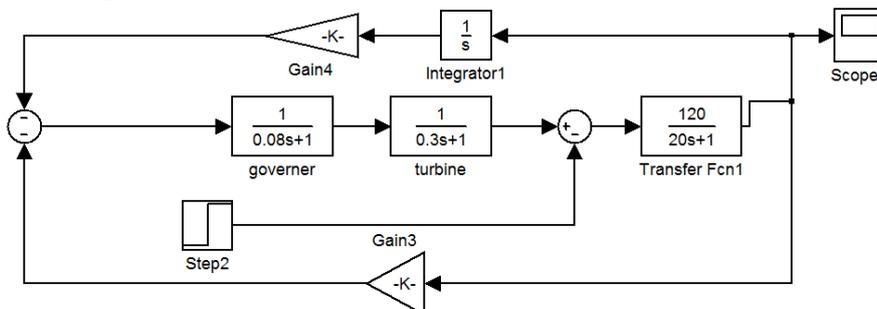
Fig 4 MATLAB Diagram of PI Controller for single Area Load Frequency Control
