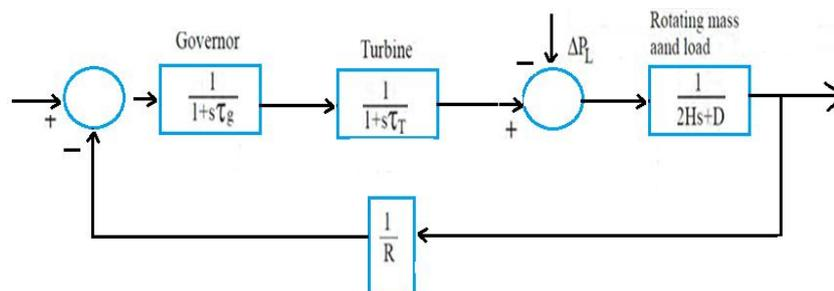
Fig1. Single-zone power system block diagram
