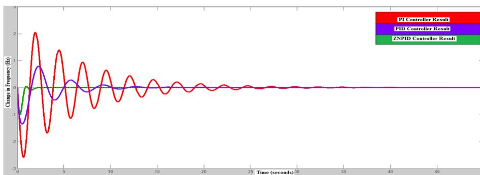
**Fig 10 frequency response of conventional PI, PID and ZN-PID controller**
