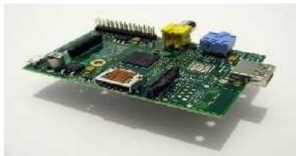
The Raspberry Pi has a Broadcom BCM2835 system on a chip (SoC), which includes an ARM1176JZF-S 700 MHz processor, Video Core IV GPU, and was originally shipped with 256 megabytes of RAM, later upgraded to 512 MB. It does not include a built-in hard disk or solid-state drive, but uses an SD card for booting and persistent storage.
