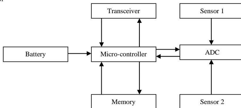
*Figure 1 : A typical architecture of the sensor node*
