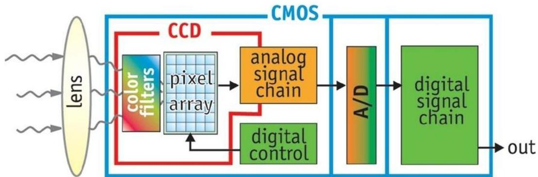
*Figure 8. Difference in Chipset Structure between CMOS Image Sensor and CCD Image Sensor*
