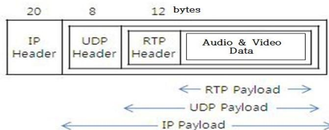
**Figure 7. RTP Stack Configuration**
