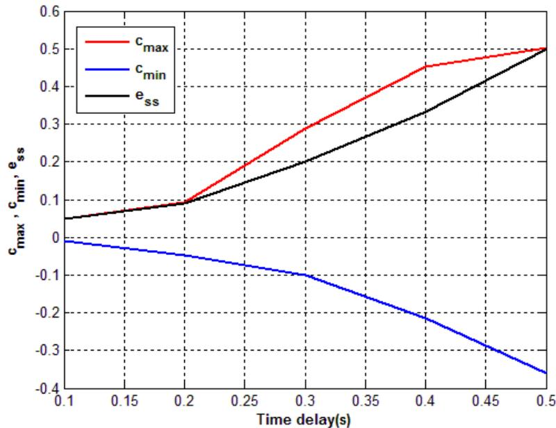
*Figure 4. Effect of time delay on  $c_{max}$ ,  $c_{min}$  and  $e_{ss}$ .*
