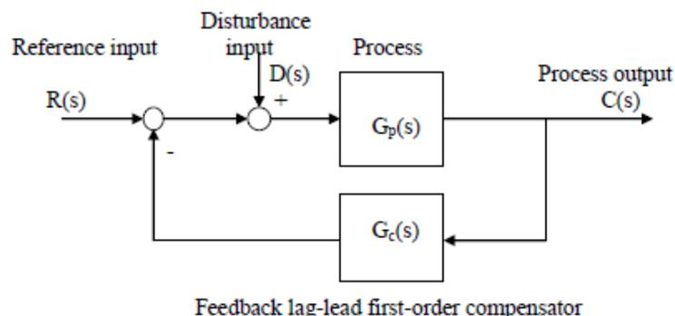
Figure 1. Control system with feedback lag-lead first-order compensator.
