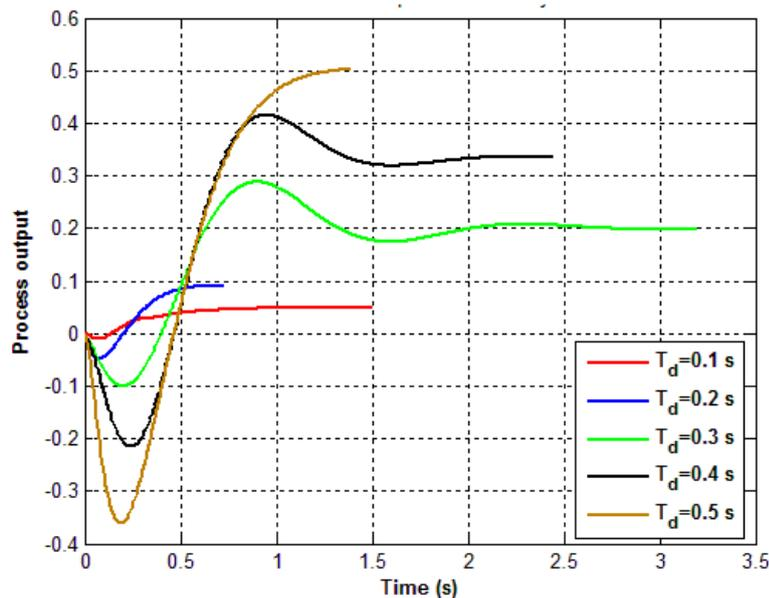
Figure 3. Effect of time delay on control system time response.
