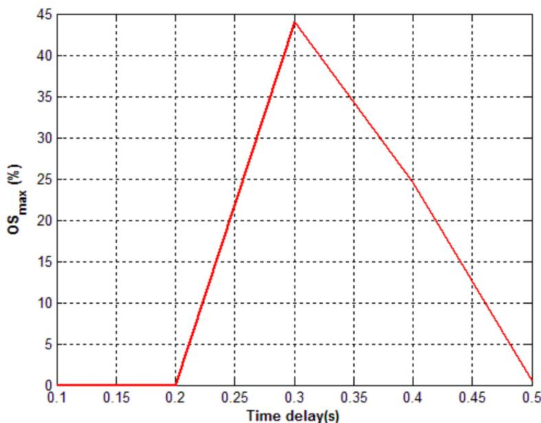
*Figure 5. Effect of time delay on  $OS_{max}$ .*
