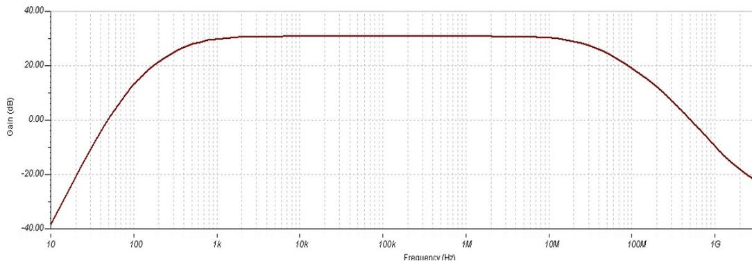
Fig 6: Frequency response of three stage amplifier
