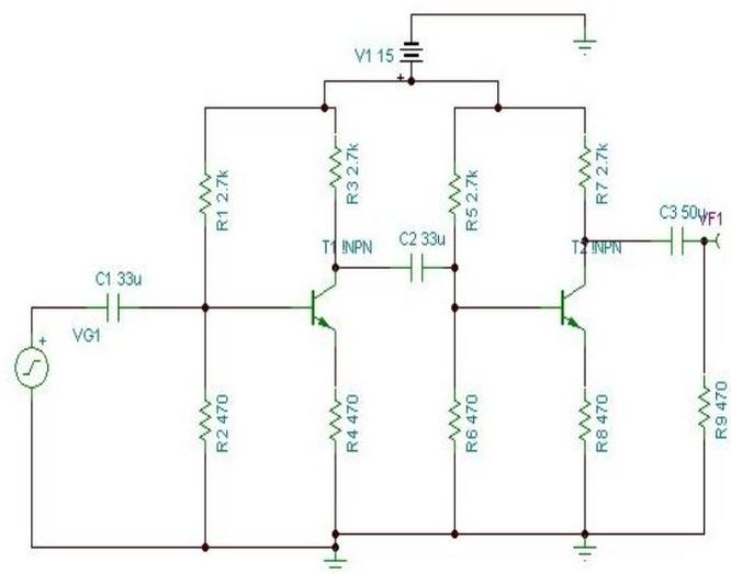
*Fig 2. Double stage amplifier*
