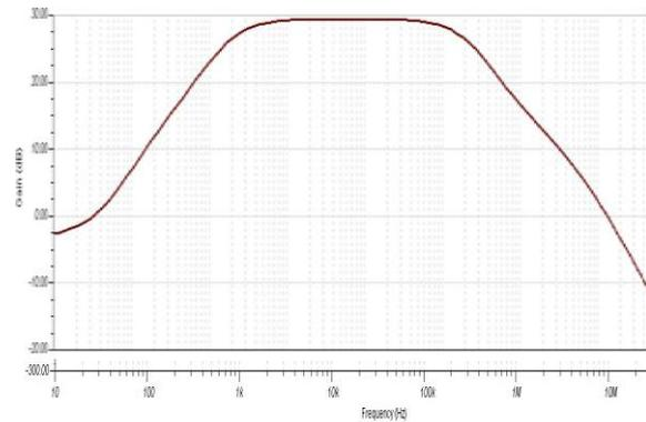
Fig 5: Frequency response of double stage amplifier
