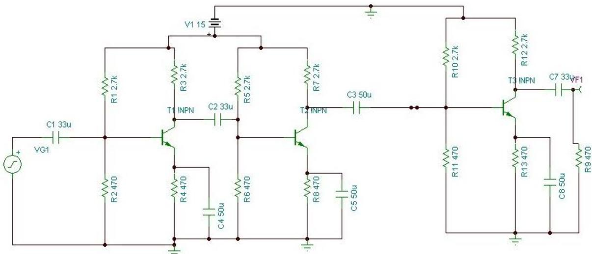
**Fig 3. Three stage amplifier**
