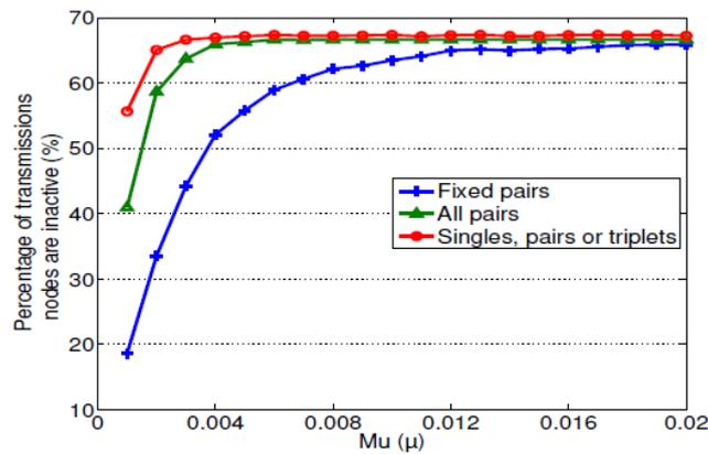
*Fig.1.6 Node inactivity for varying channel quality*
