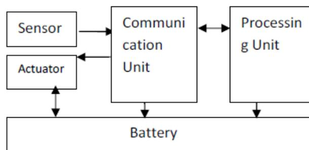
Figure 1.4 Structure of a sensor node
