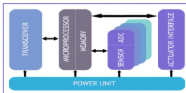
Figure 1.2 Architecture of Sensor Node
