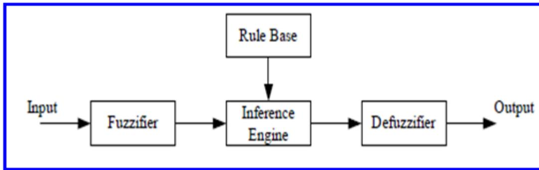
*Fig 2 main Components of fuzzy logic controller*
