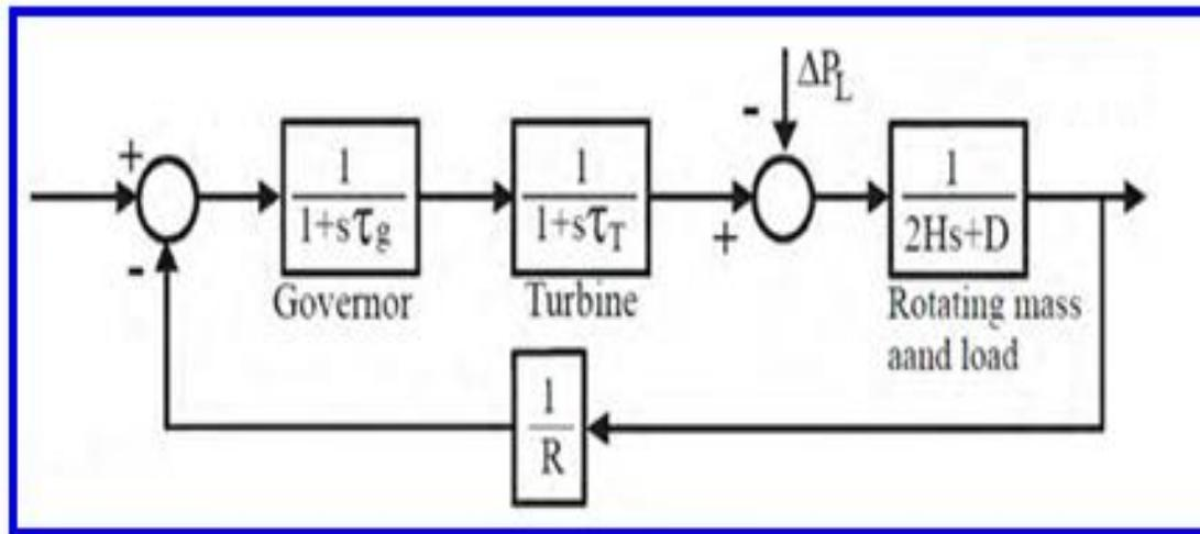
Fig.1. Automatic Load Frequency Control single area power system
