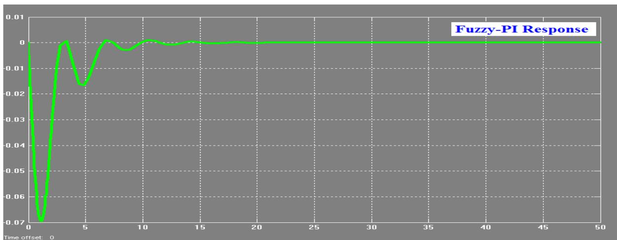
Fig 12 Frequency response of single area with fuzzy- Proportional Integral controller
