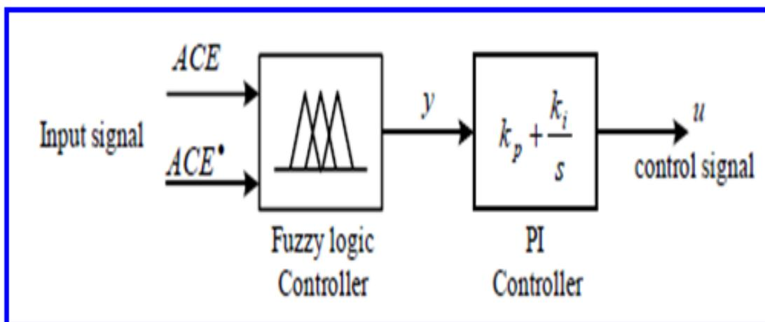
*Fig 3 fuzzy logic proportional integral controller (FL-PI).*
