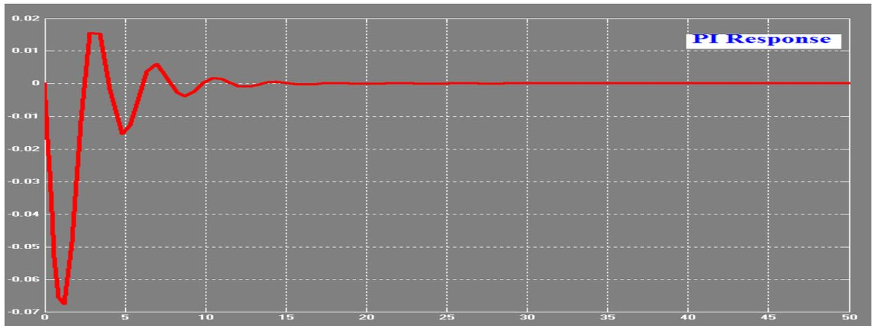
Fig 10 Frequency response of single area with Proportional Integral controller
