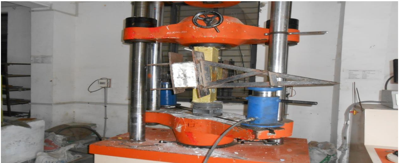
Fig.9 Twisted shape of the Beam-Column Joint No.W1
