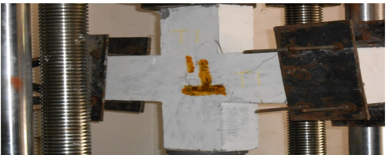
Fig.8 Beam-Column Joint No. T1 after cracking
