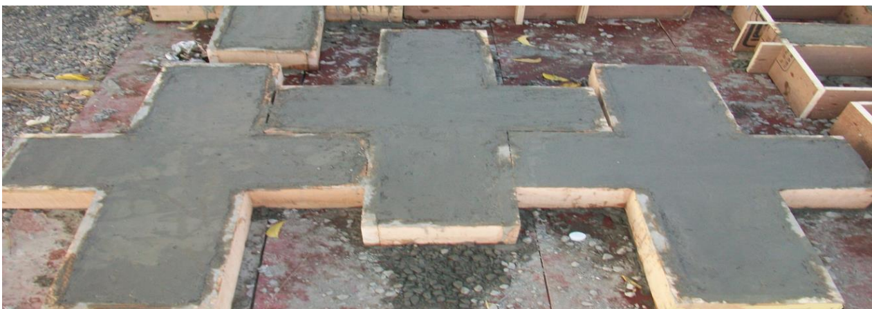
Fig.2 Casting Beam-Column Joint Specimen
