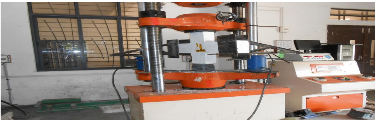
Fig.5 Experimental for Beam-Column Joint Design For Torsion No.T1
