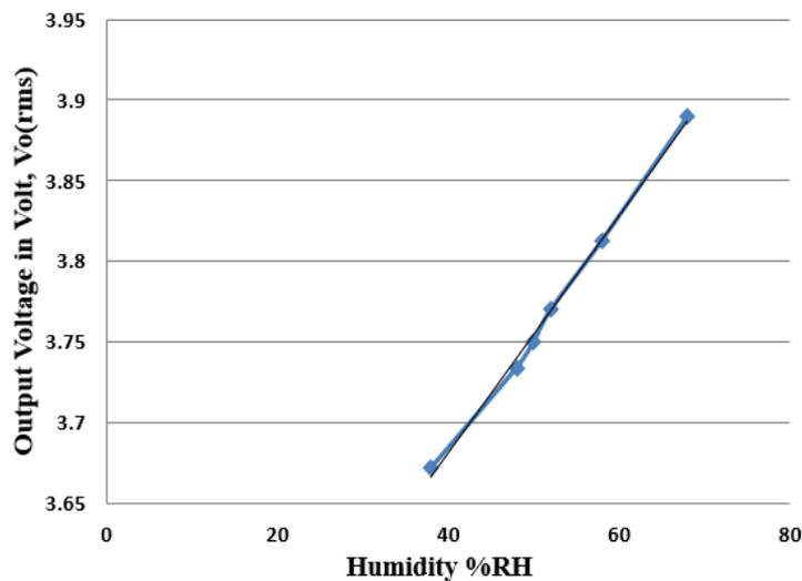
Fig. 9. Humidity Vs Voltage after Amplification
