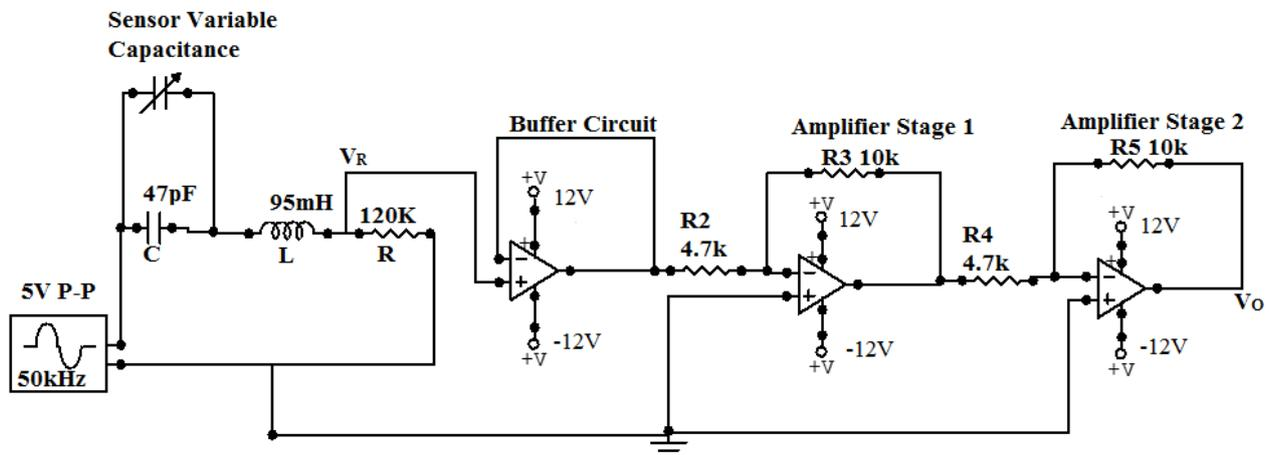
Fig. 4. Signal conditioning circuit for semi cylindrical capacitive sensor.
