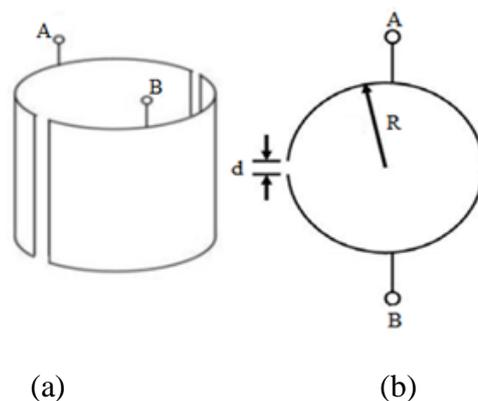
Fig. 1. (a) Architecture of semi-cylindrical capacitive sensor. (b) Top view of semi-cylindrical capacitive sensor.
