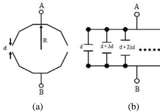
Fig. 2. (a) Approximate structure of the semi-cylindrical capacitive sensor without dielectric for numerical analysis method. (b) Equivalent capacitors between A and B terminals of semi cylindrical plates.
