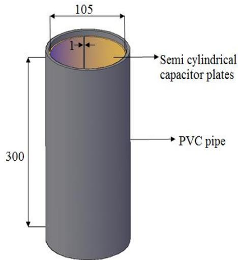
Fig. 3. Isometric view of semi cylindrical capacitive humidity sensor (All dimensions are in mm).
