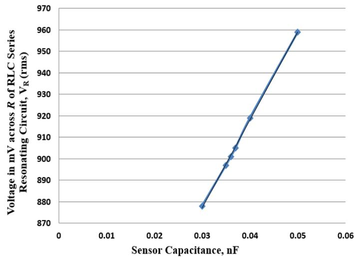
*Fig. 7. Sensor Capacitance Vs Voltage across R*
