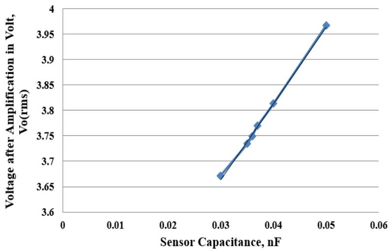
*Fig. 8. Sensor Capacitance Vs Voltage after Amplification*
