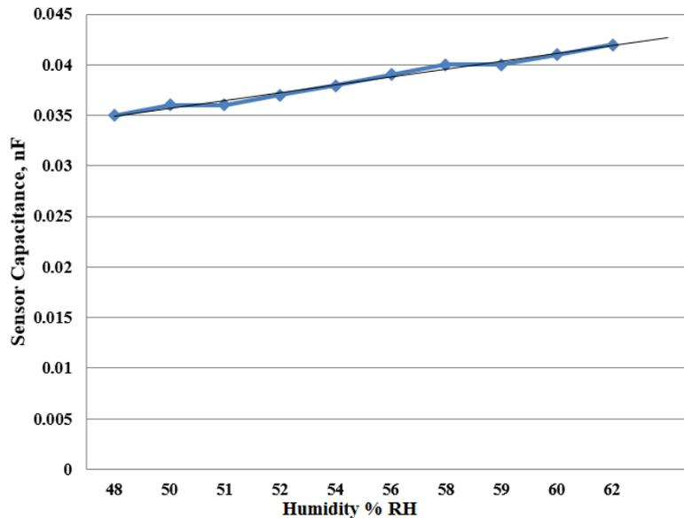
**Fig. 5. Humidity Vs Capacitance Graph**
