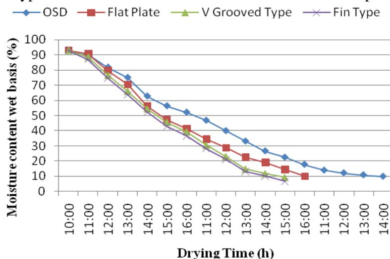
Figure: 5 Variation of moisture (%) against drying time in different dryers for tomato drying
