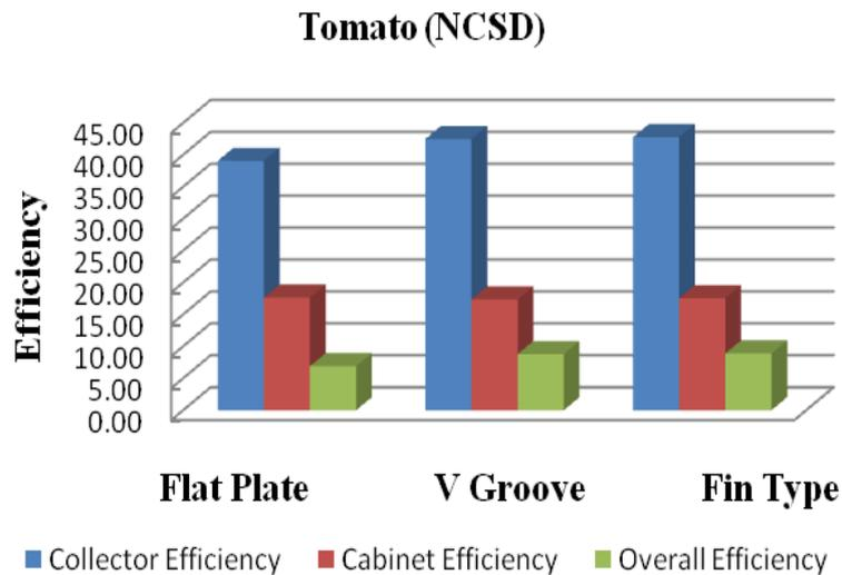
*Figure: 6 Comparison of collector, cabinet, overall efficiencies of different dryers for tomato drying*
