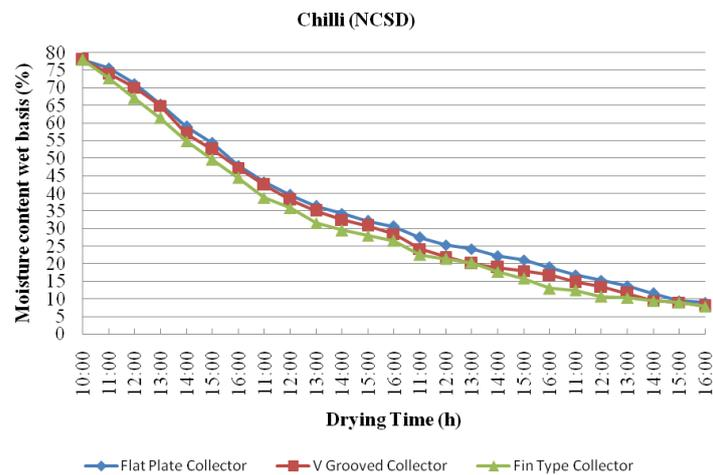
Figure: 8 Variation of moisture (%) against drying time in different dryers for chilli drying
