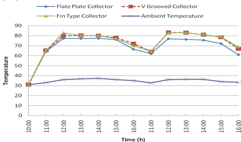
Figure: 3 Variation of collector outlet temperature against drying time for tomato drying by natural convection
