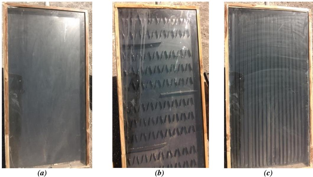
(a) Flat Plate (b) Fin Type Plate (c) V-Groove Type
