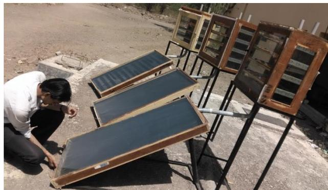
*Figure: 1 Pictorial View of Fin, Flat-Plate, V-Groove Type Collectors Integrated With Separate Cabinet.*
