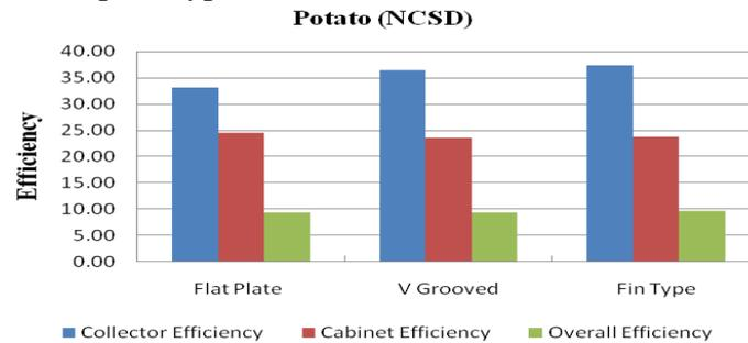
**Figure: 11 Comparison of Collector, Cabinet, Overall Efficiencies of Different Dryers for Natural Convection Potato Drying.**
