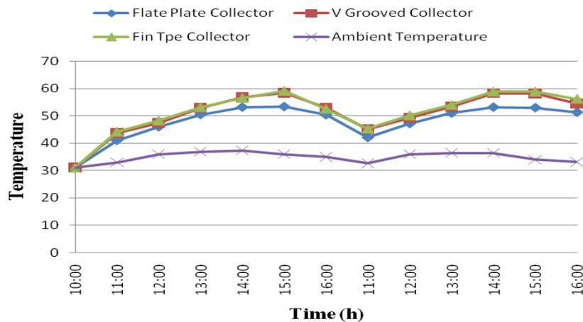
Figure: 4 Variation of cabinet temperature against drying time for tomato drying
