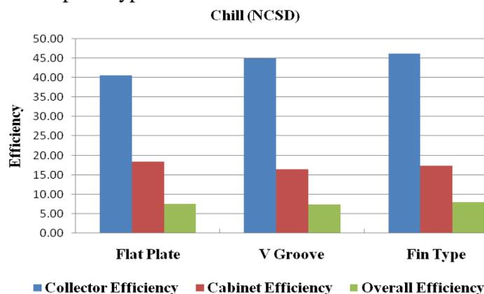
Figure: 9 Comparison of collector, cabinet, overall efficiencies of different dryers for natural convection chilli drying
