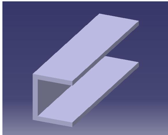
*Figure 4: Solid model design of column with C-cross sectional shape in CATIA V5 software*
