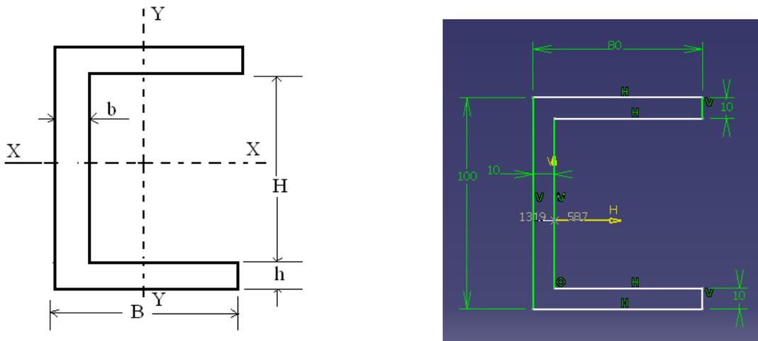
*Figure 3: Cross sectional view of the column with C-cross sectional shape*
