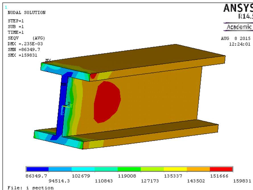
*Figure 7: Stress contour for the I-section column*
