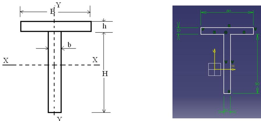
*Figure 5: Cross sectional view of the column with T-cross sectional shape*
