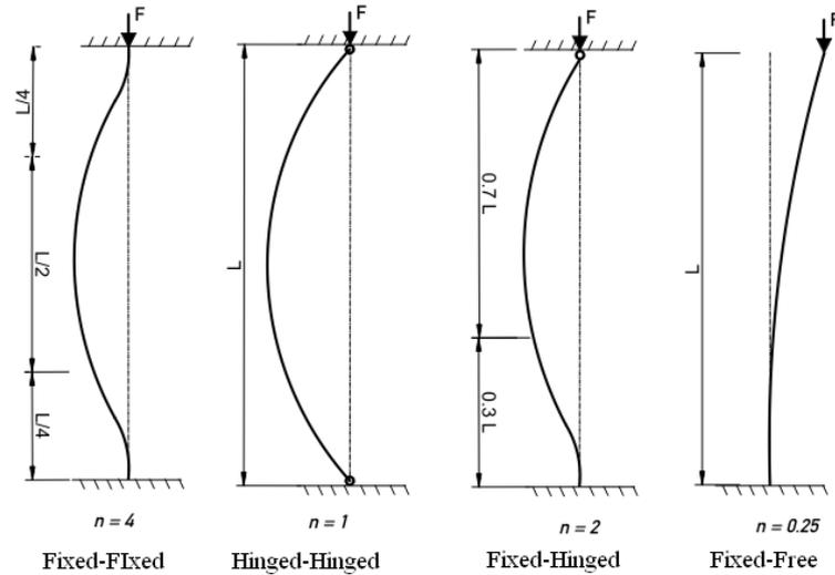
**Figure 1: Column with different end conditions**
