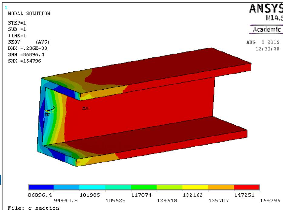
*Figure 8: Stress contour for the C-section column*
