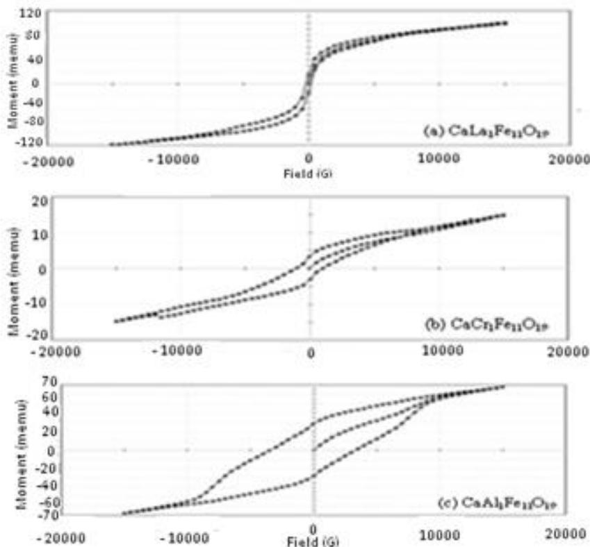
Fig.(4): Hysteresis loops for samples of synthesized Ca substituted hexaferrite of (a) CaLa<sub>1</sub>Fe<sub>11</sub>O<sub>19</sub> (b) CaCr<sub>1</sub>Fe<sub>11</sub>O<sub>19</sub> (c) CaAl<sub>1</sub>Fe<sub>11</sub>O<sub>19</sub>
