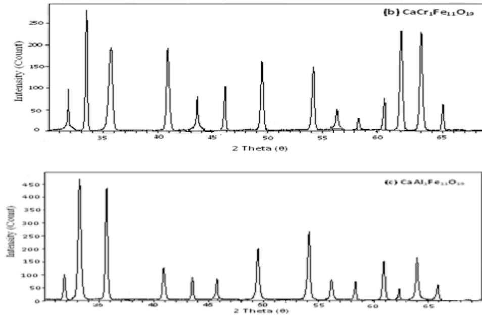
Fig.(1): XRD Pattern of synthesized Ca Substituted Hexaferrite
