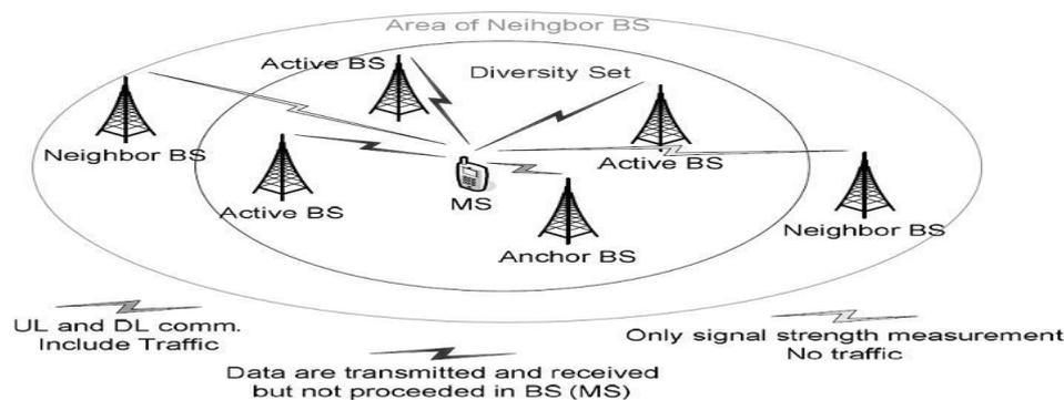
**Figure 2.2.3. Fast Base Station Switching Handover [3]**
