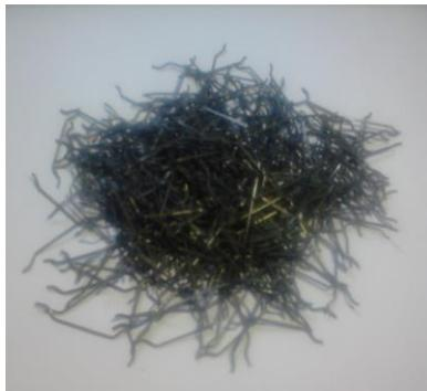
Figure 3. Hooked end steel fiber.
