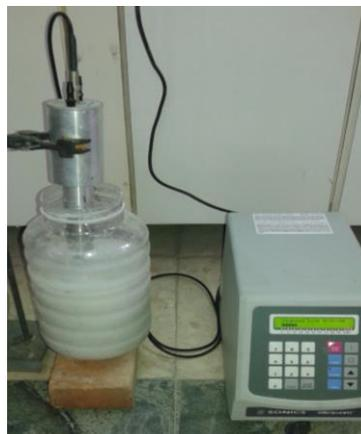
Figure 4. Ultra-sonication probe.
