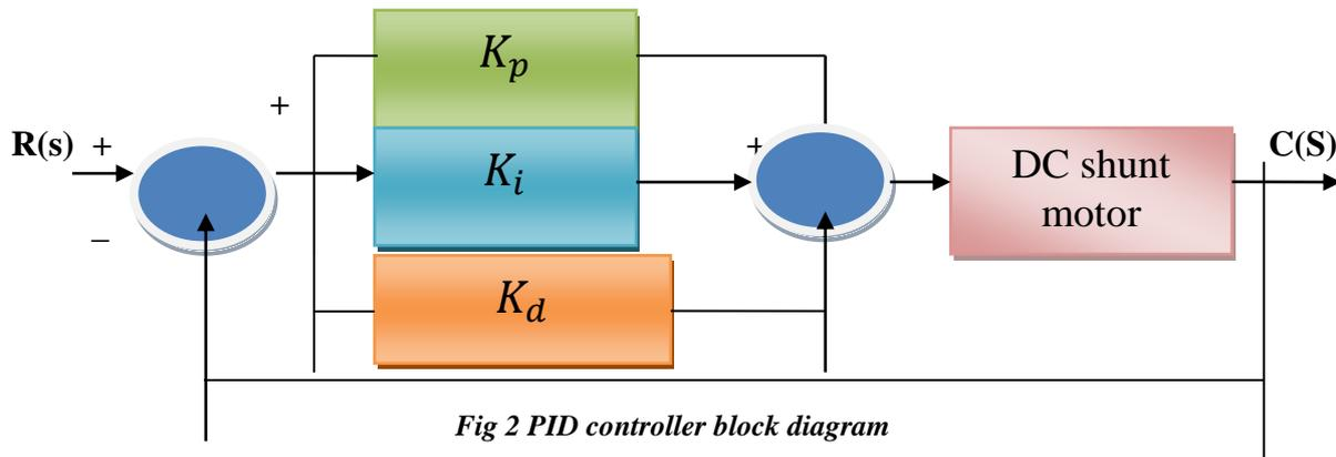
*Fig 2 PID controller block diagram*
