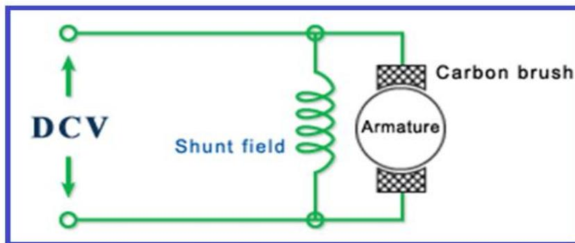
*Fig 1. Model Of DC Shunt Motor*
