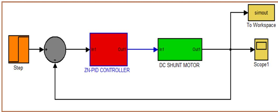
Fig 3 Simulink model of ZN controller with PID controller
