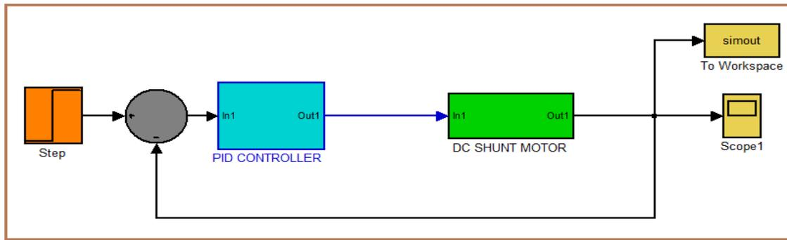
*Fig 8 PID-MATLAB Simulink Model*
