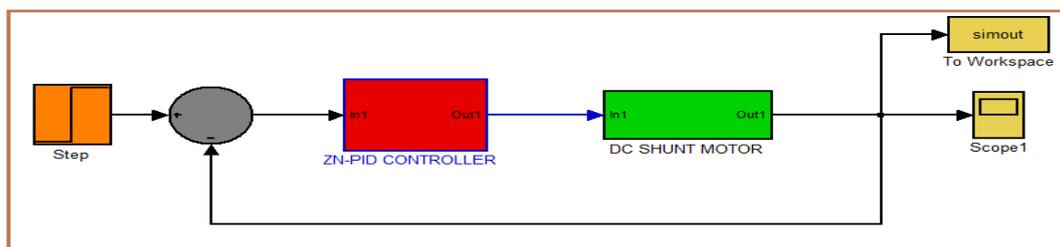
*Fig 10 MATLAB simulink model of dc shunt motor*
