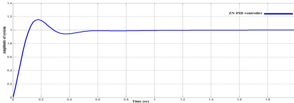
Fig 11 best graph of ZN-PID Controller
