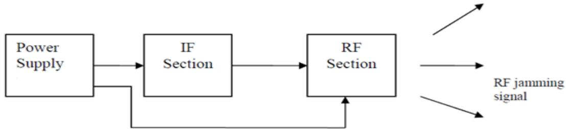
Figure 1. Block diagram of working of Mobile Jammer.
