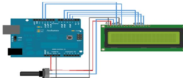
**Fig 3.3: LCD – Arduino Interface Circuit**
