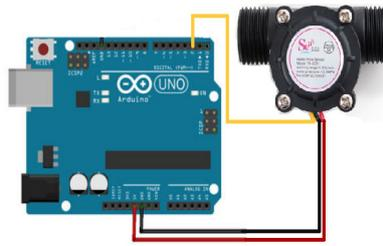
**Fig 3.1: Flow sensor – Arduino Interface circuit.**
