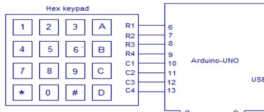
**Fig 3.4: Keypad Arduino Interface**
