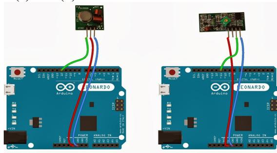
**(a) Arduino- RF TX (b) Arduino- RF RX**
