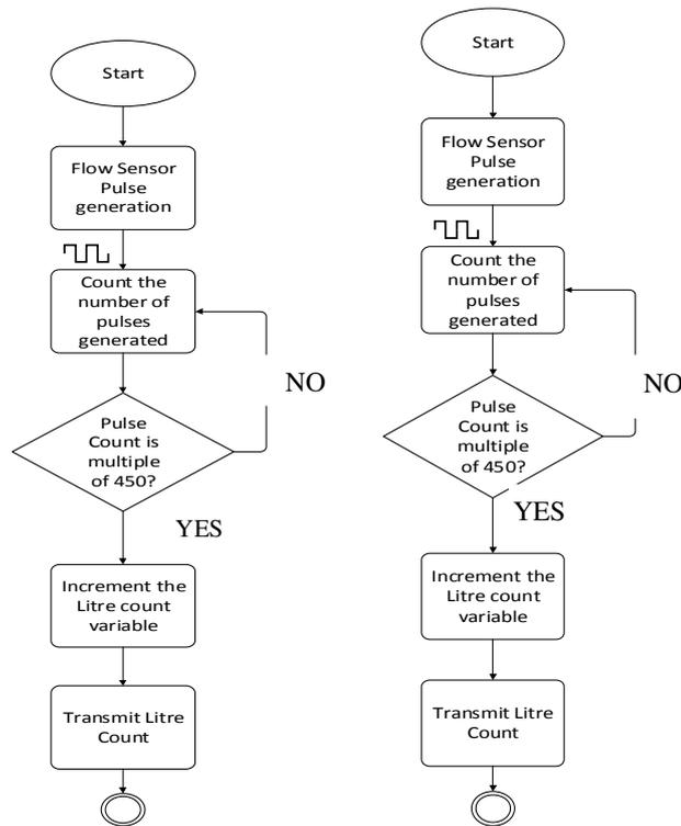
Fig 3.5: transmitter section
