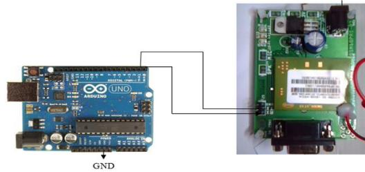
**Fig 3.3: GSM-Arduino interface circuit**
