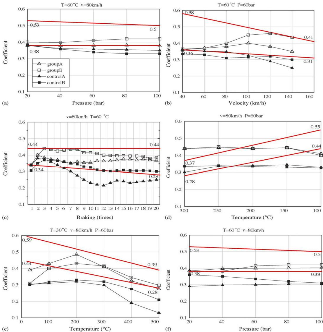
Fig. 2. Dynamometer test results of disc brake pads modified with nano powdered rubber, VP-402.
