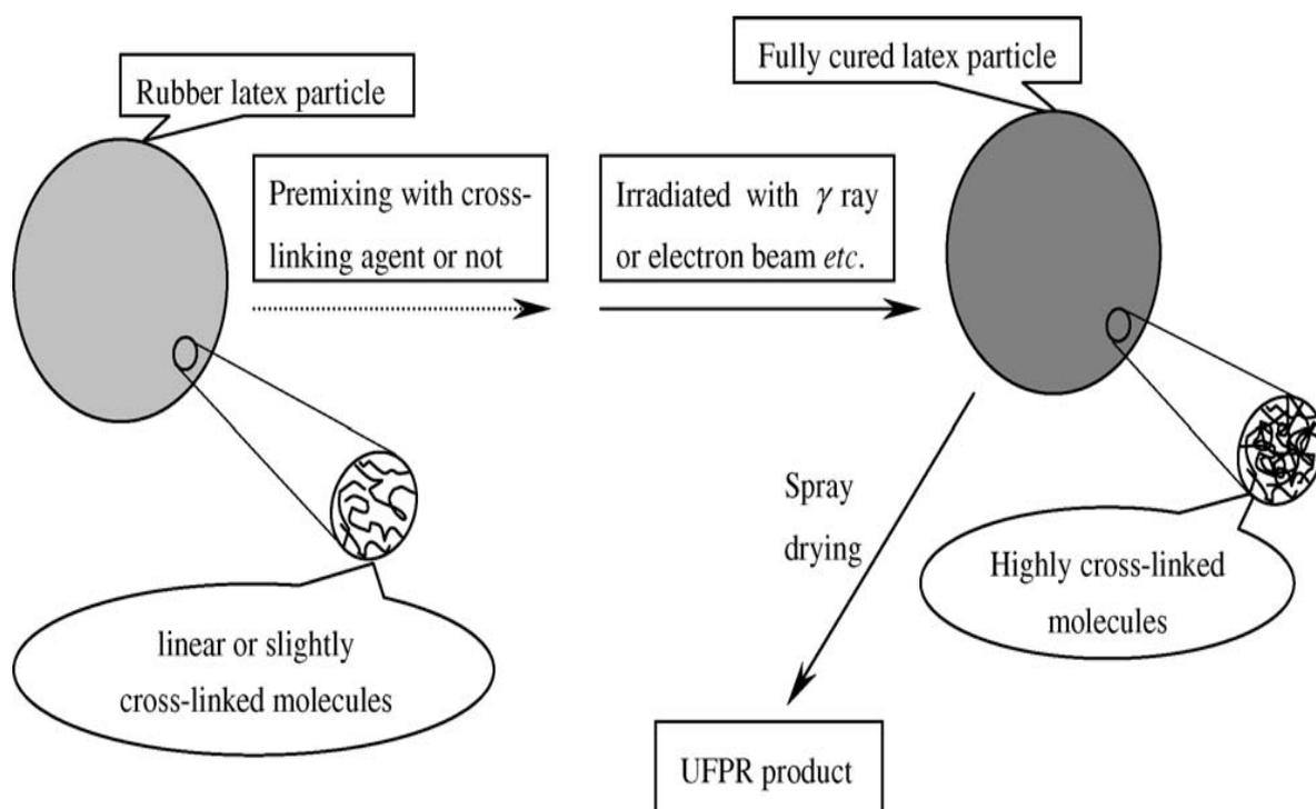
Figure 1. Schematic diagram of the preparation of UFPR
