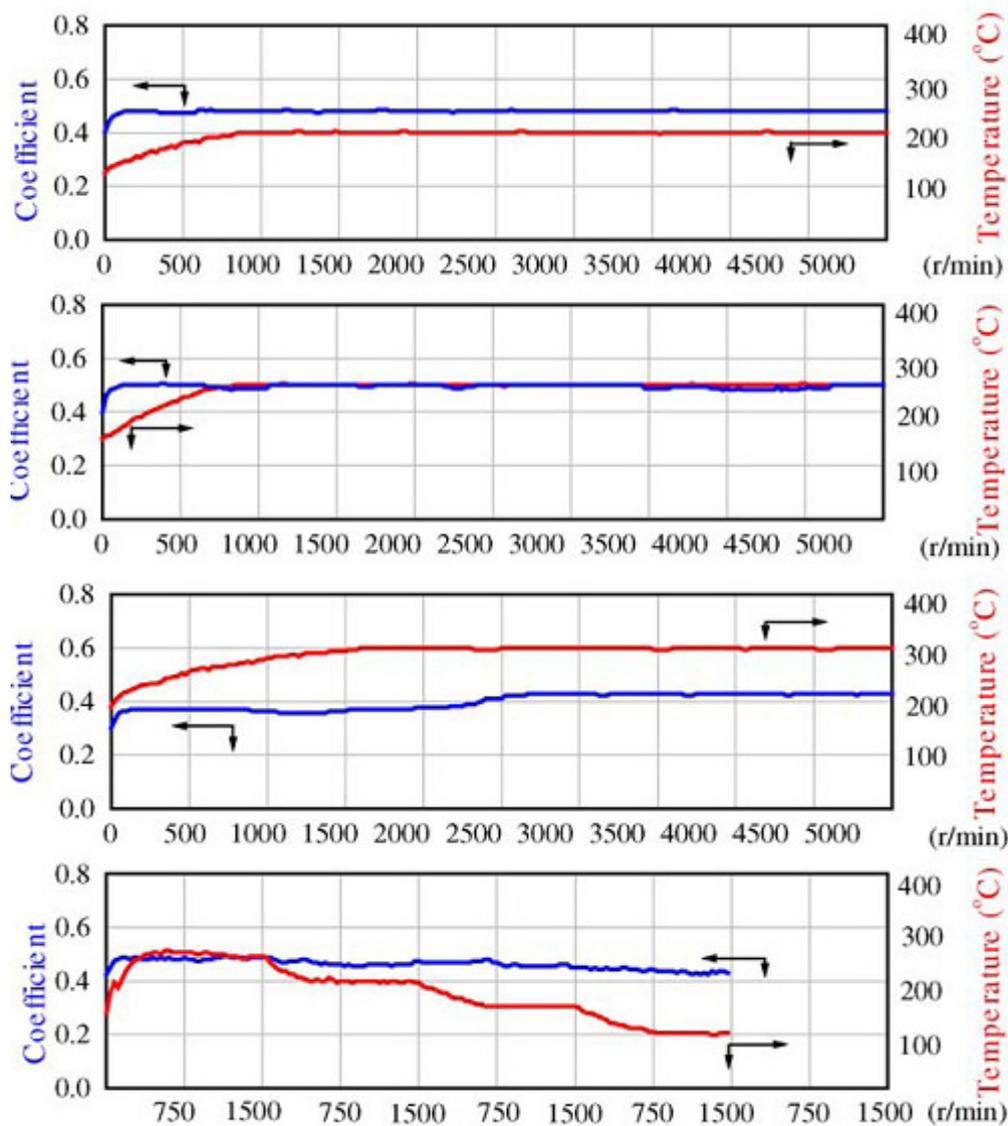
Figure 3. Friction test result of clutch facings modified with nano powdered rubber VP-401 according to GB 5764/98 standard.
