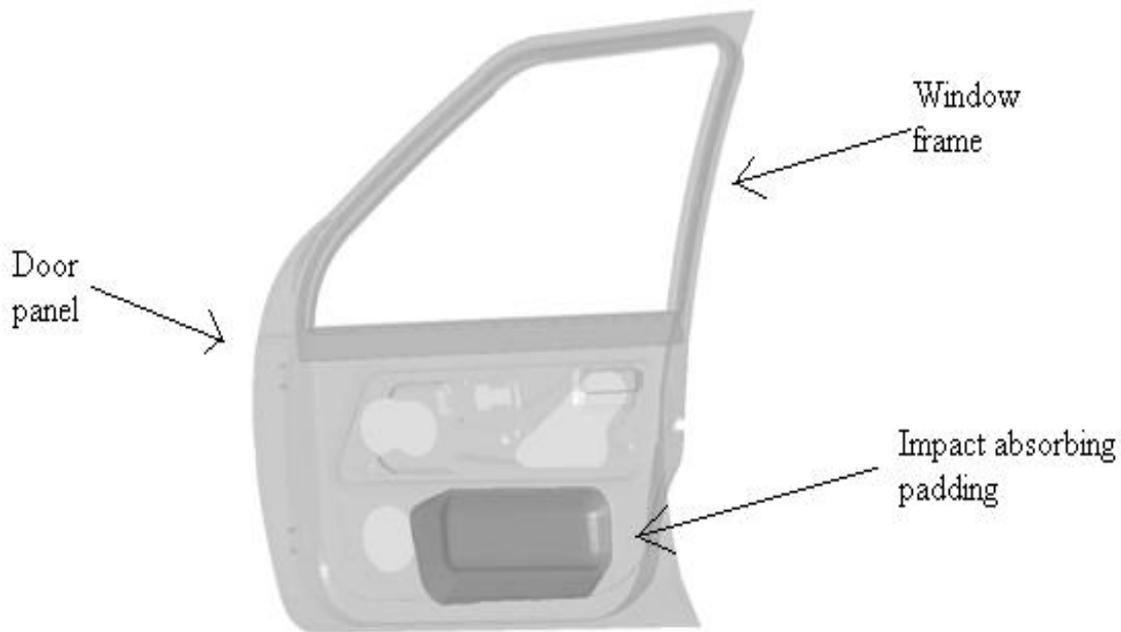
*Figure 1: Inclusion and position of the protection padding [16]*
