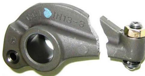
*Fig.2. Failure of a rocker arm at neck*
