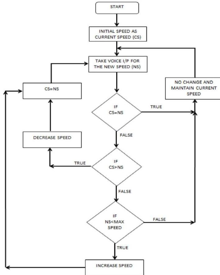
Fig 4.1: Flowchart of the voice controlled speed system
