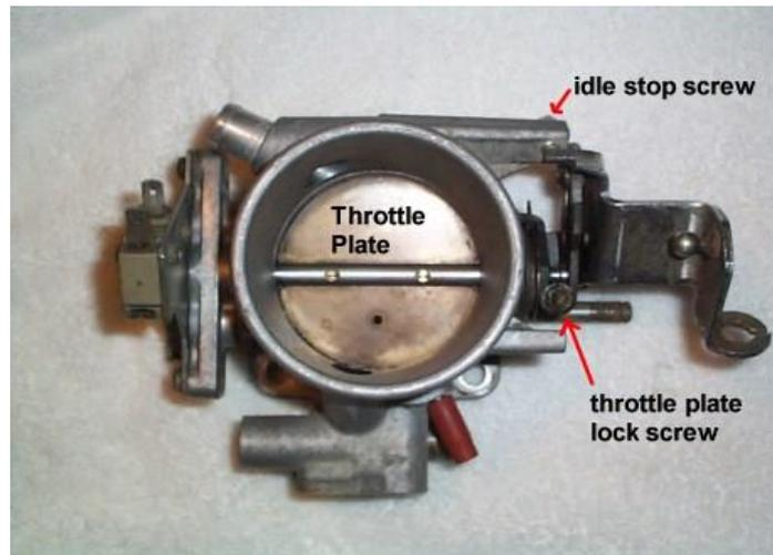
Fig 2.3: View of the throttle body
