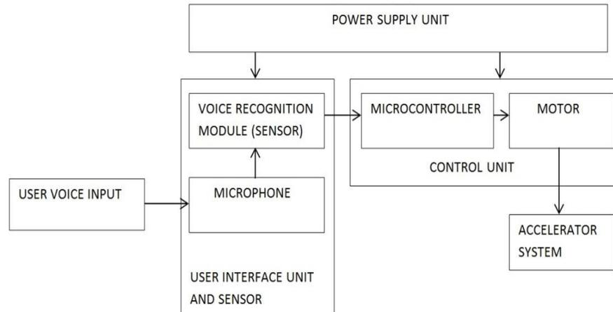
Fig 3.1: Block diagram of Voice Controlled Speed System
