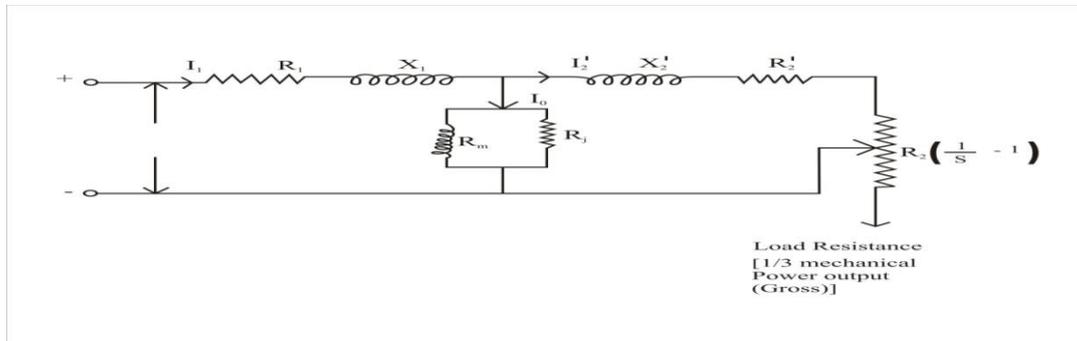
Equivalent circuit diagram of a three phase induction machine
