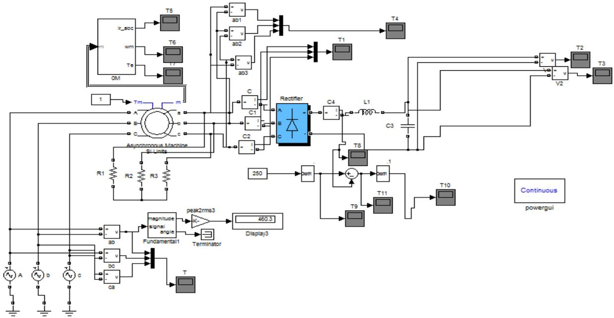
Figure. Matlab simulation of three phase induction machine
