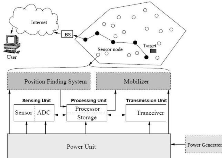
**Figure 1.1: Communication Architecture of Wireless Sensor Networks**
