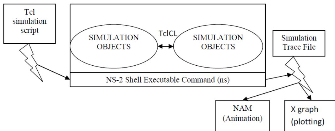
*Figure 5.1: Basic Architecture Of Ns-2*
