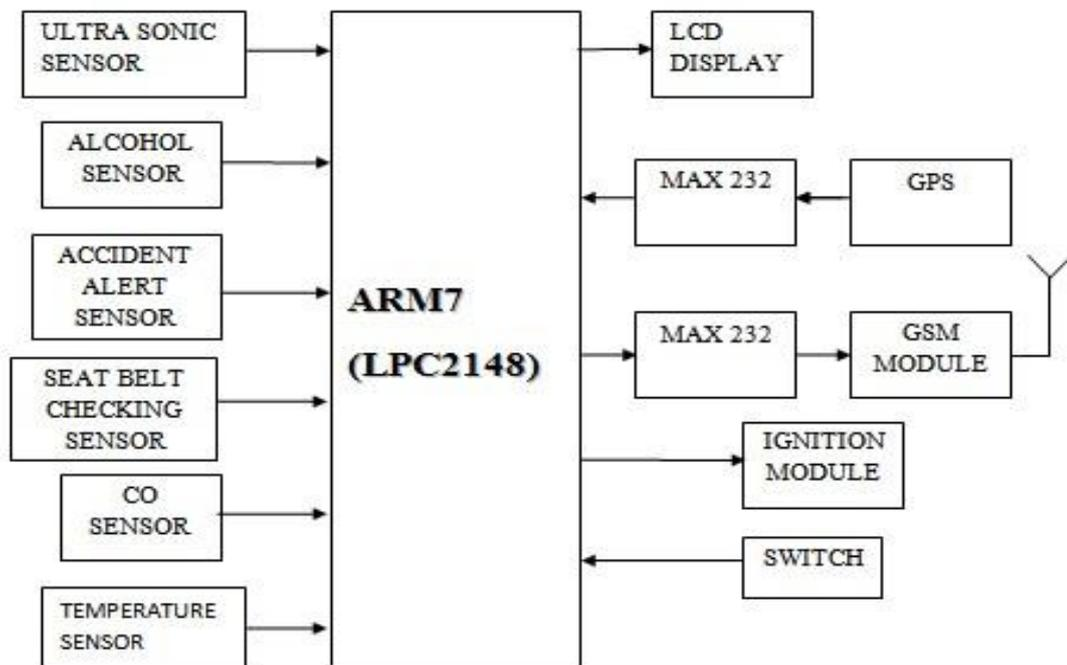
Fig 1: Block Diagram
