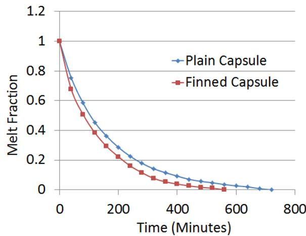
**Figure 8. Comparison of plain and finned capsule for HTF temp  $-2^{\circ}\text{C}$  and flow rate 3 LPM.**
