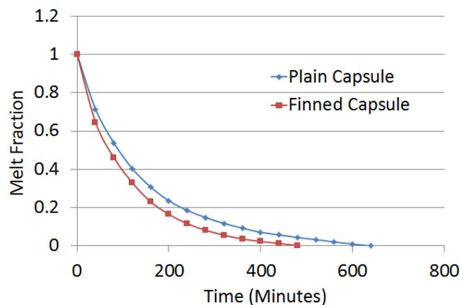
**Figure 9. Comparison of plain and finned capsule for HTF temp  $-7^{\circ}\text{C}$  and flow rate 5 LPM.**
