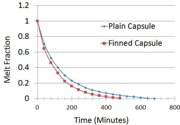
**Figure 7. Comparison of plain and finned capsule for HTF temp  $-7^{\circ}\text{C}$  and flow rate 3 LPM.**
