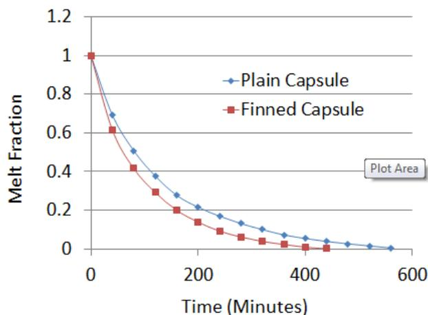
**Figure 6. Comparison of plain and finned capsule for HTF temp -120C and flow rate 3 LPM.**
