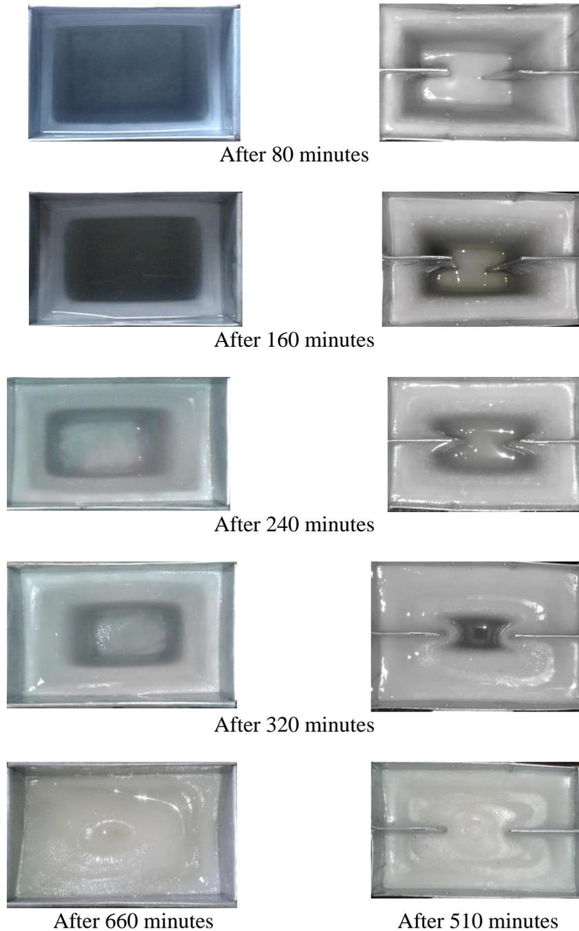
**Figure 5. Solidification images of PCM inside the capsule with HTF inlet temperature -70C and flow rate 3 LPM.**
