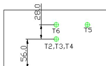
**Figure 4. Position of RTD's in finned capsule**
