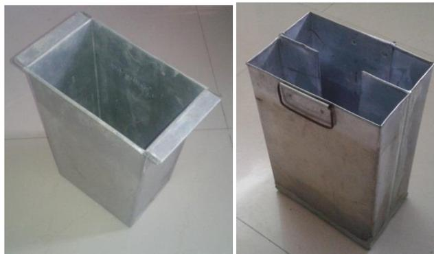
*Figure 1. G.I.capsules with and without fins*
