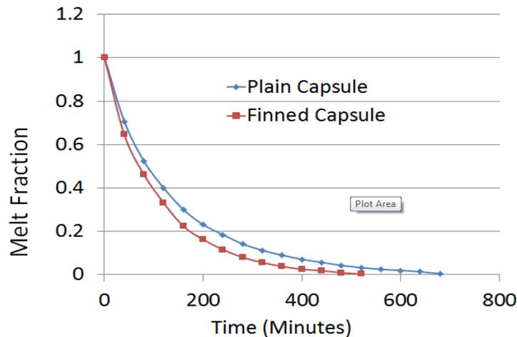
Figure 10. Comparison of plain and finned capsule for HTF temp  $-7^{\circ}\text{C}$  and flow rate 1 LPM.
