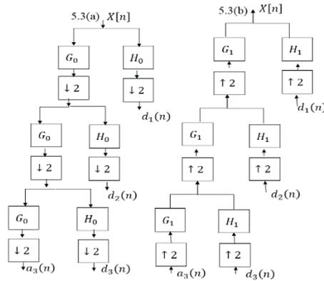
Fig 1.3(a) and (b) explains the DWT analysis filter and IDWT synthesis filter respectively.[1]
