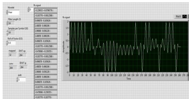
Fig. 3.3 The received signal and waveform generated for DWT OFDM
