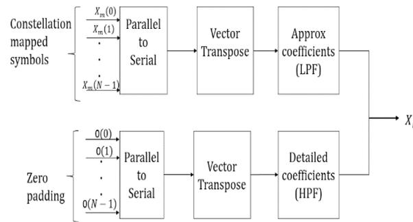
Fig 1.5 IDWT transmitter block[8], [9]
