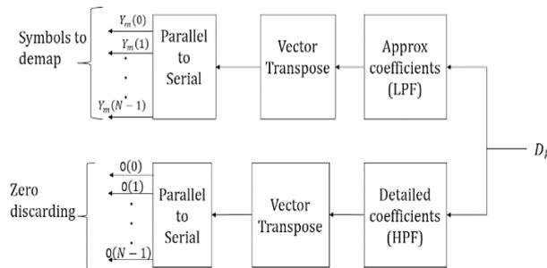
Fig 1.6 DWT receiver block[8], [9]
