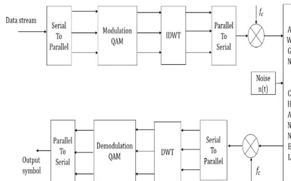
Fig 1.4 proposed DWT OFDM system model[6], [7]
