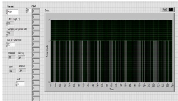
Fig 3.1 shows the input waveform generated for the random bit sequence.
