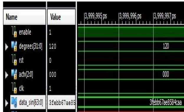
Fig.9: Simulation results of double precision floating point Sine function
