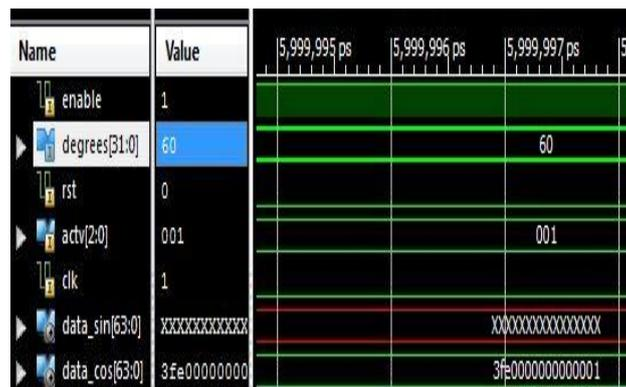
Fig.10: Simulation results of double precision floating point Cosine function
