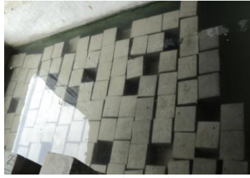
Figure 10. Cube curing tank
