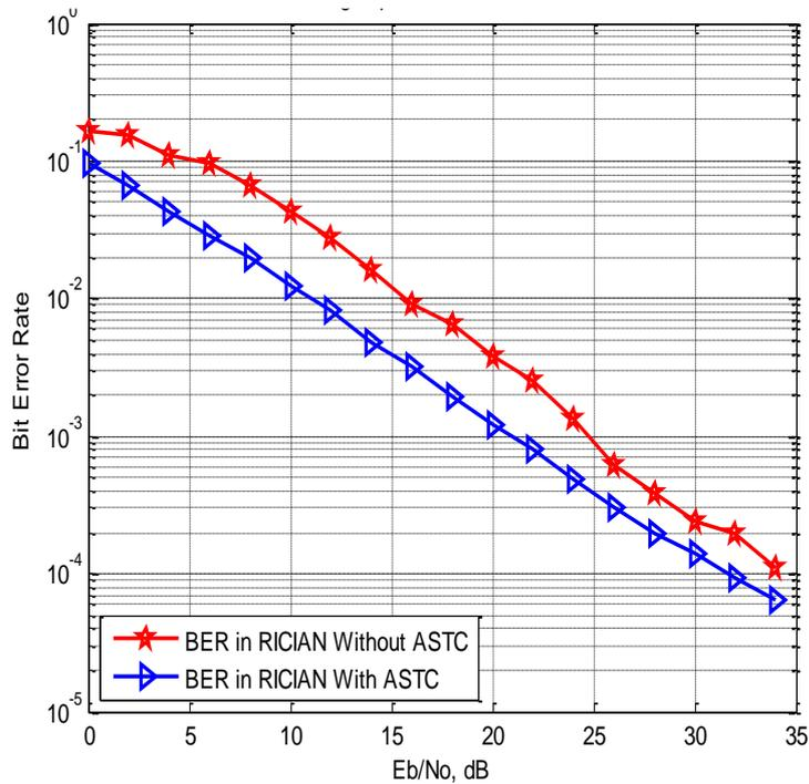
Fig:3 BER Comparison for Rician with or without ASTC Encoder.
