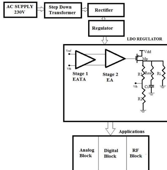
Fig. 1. Power Supply Section Using Proposed LDO.
