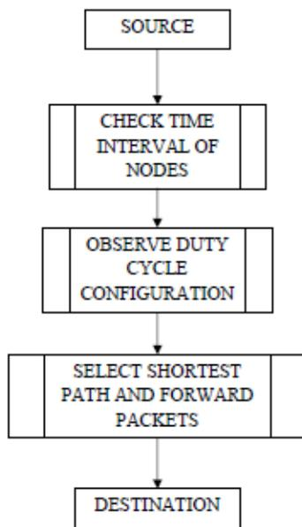
Figure 4. Data Flow Diagram of Dynamic Route Maintenance Module
