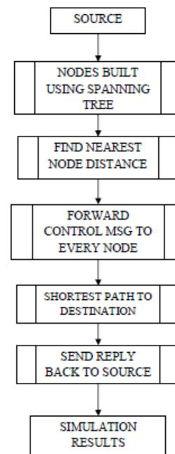
Figure 5. Data Flow Diagram of Route Updating modules
