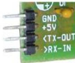
Figure6. Pins of PLC Modem: 1187
