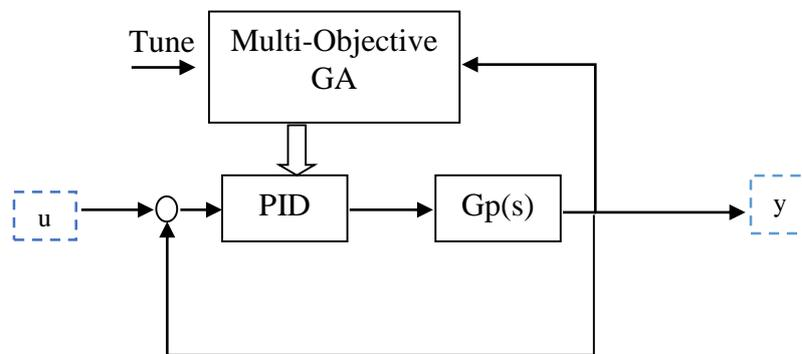
**Fig 1:** Block Diagram of Multi-Objective GA PID
