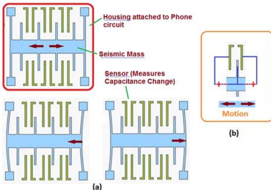
The figure (b), a cutout of figure (a), shows change in capacitance as a result of change in position of Seismic mass, when smart device is tilted or changed in orientation. This will recognize the change
