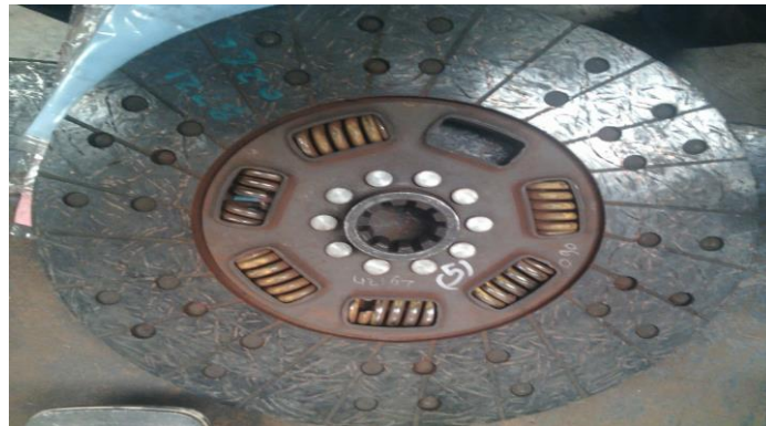
Fig.2: Photo of 310 D.P.A (damper spring broken)
