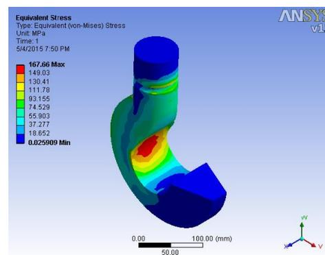
Figure 9. Stress pattern for trapezoidal cross-section
