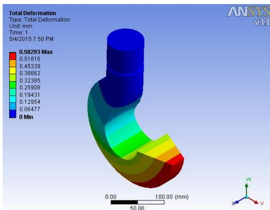
*Figure 24. Total deformation plot for basic cross-section*
