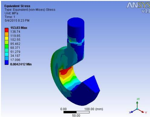
Figure 12. Stress pattern for iteration No. 1
