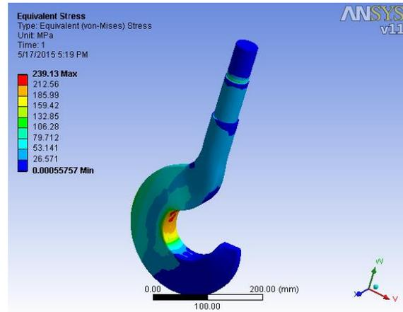
*Figure 23. Stress pattern for optimized cross-section*
