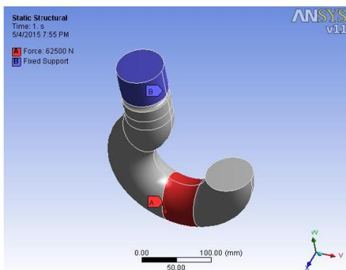
*Figure 4. Sketch showing Boundary conditions for circular cross-section*
