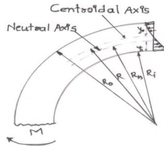
Figure 2. Hyperbolic stress distribution in curved beam
