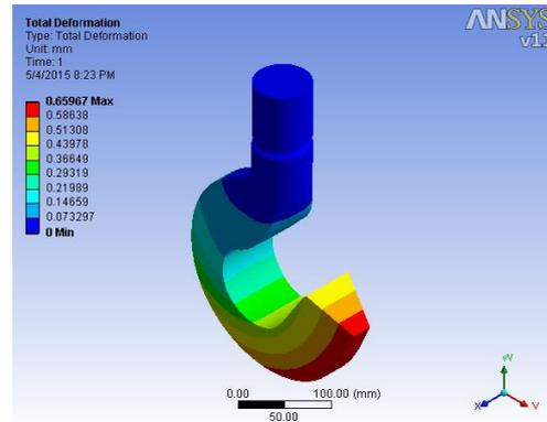
Figure 13. Total deformation values for iteration No. 1
