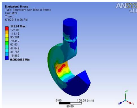
Figure 14. Stress pattern for iteration No. 2
