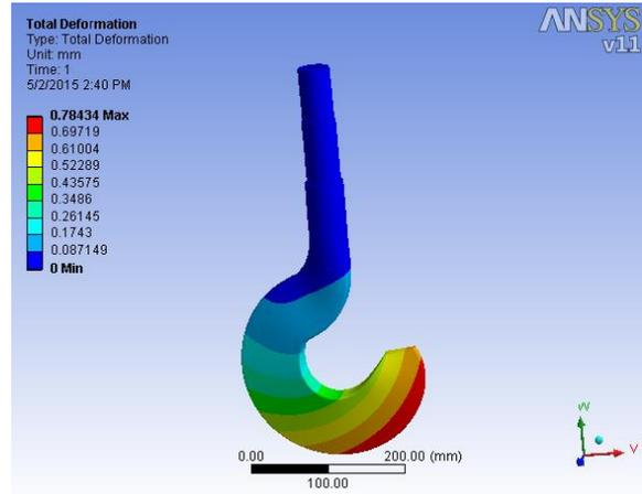
Figure 19. Total deformation pattern for iteration No. 4
