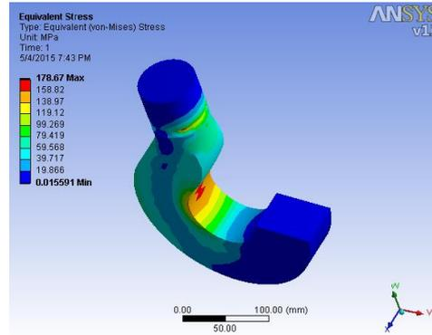
Figure 7. Stress pattern for rectangular cross-section
