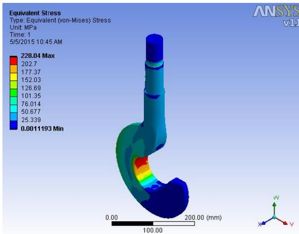
Figure 20. Stress pattern for iteration No. 5
