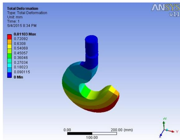
Figure 17. Total deformation pattern for iteration No. 3
