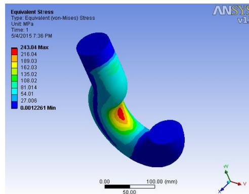
*Figure 5. Stress pattern for circular cross-section
