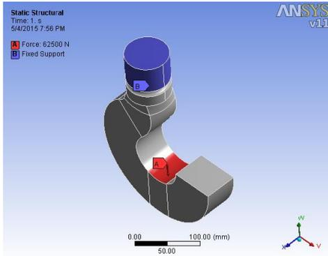
Figure 6. Sketch showing Boundary conditions for rectangular cross-section
