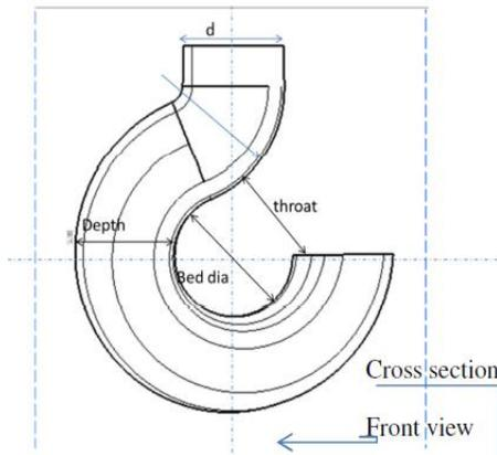
Figure 1. Sketch showing crane hook notations
