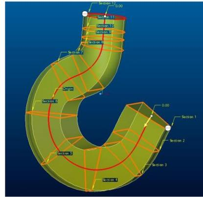
**Figure 10.** Sketch shows hook portion for shape optimization **Figure 11.** Sketch showing location for twelve c/s
