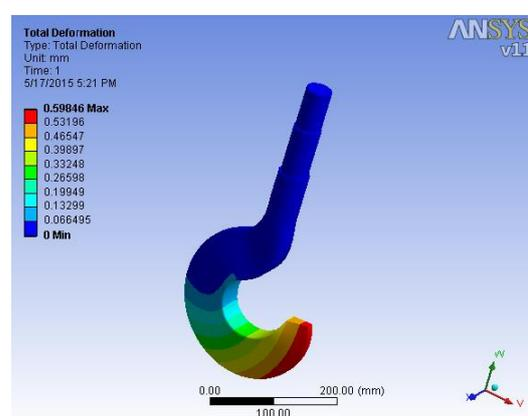
*Figure 25. Total deformation plot for optimized cross-section*
