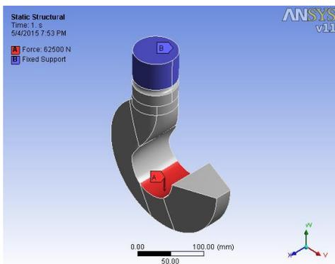
Figure 8. Sketch showing Boundary conditions for trapezoidal cross-section
