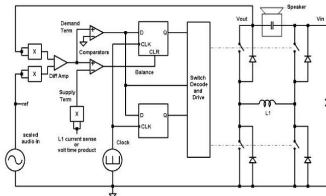
Fig.2 Circuit diagram of a switched-mode assisted linear power amplifier.
