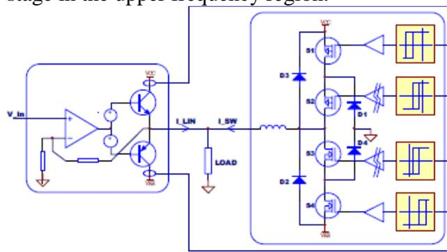
Fig5 : three level NPC switching level
