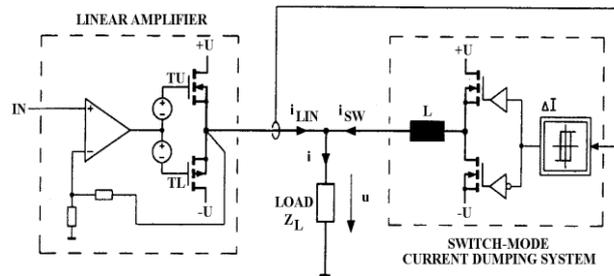
Fig. 1 Simplified circuit diagram of a linear power amplifier
