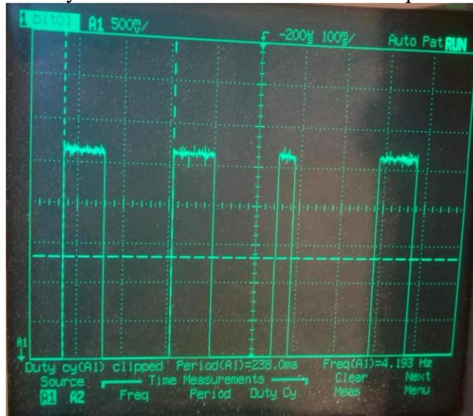
**Fig. 7 Output Pulses at pin CF in ADE7751 when a 100 W LOAD is Connected**
