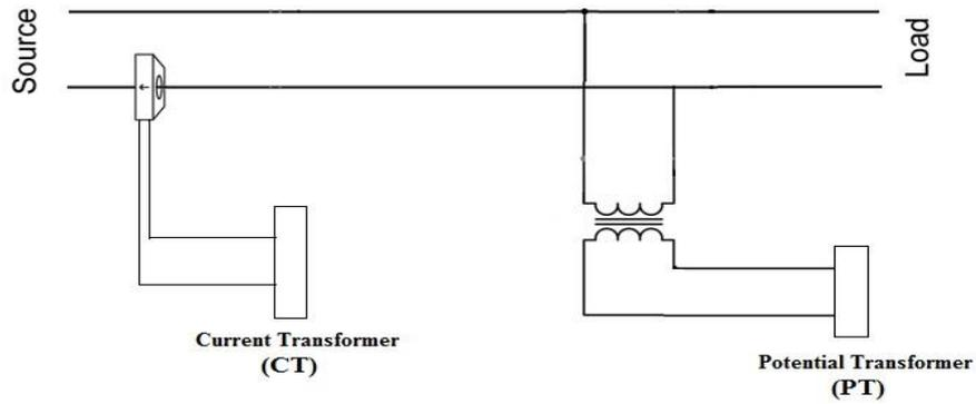
Fig. 6 CT-PT connection Diagram
