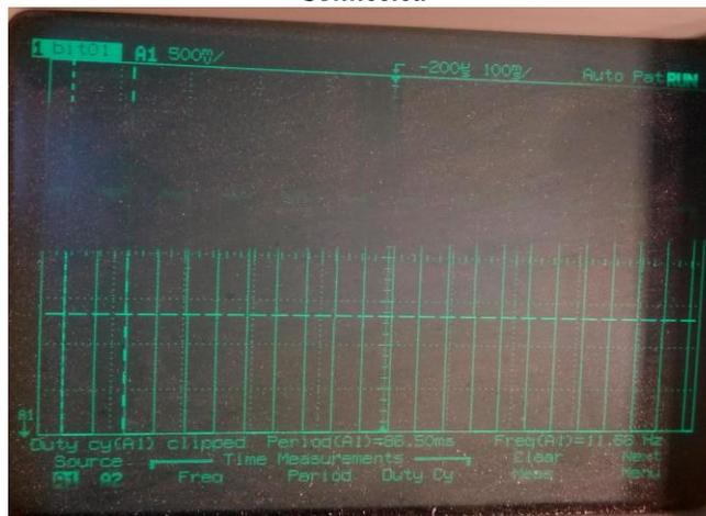
**Fig. 8 Output Pulses at pin CF in ADE7751 when a 300 W LOAD is Connected**
