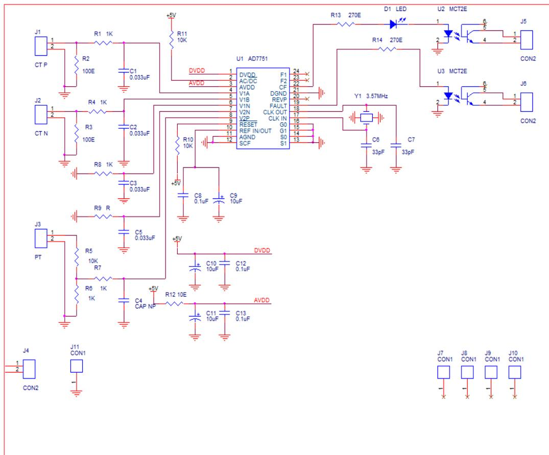
Fig.6 Circuit for energy meter.
