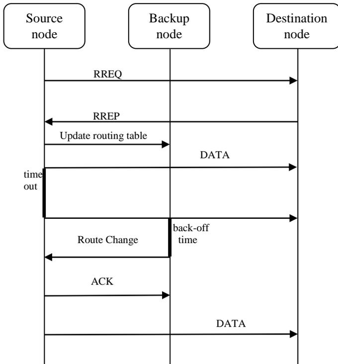
Fig.2 Sequence diagram of route recover process
