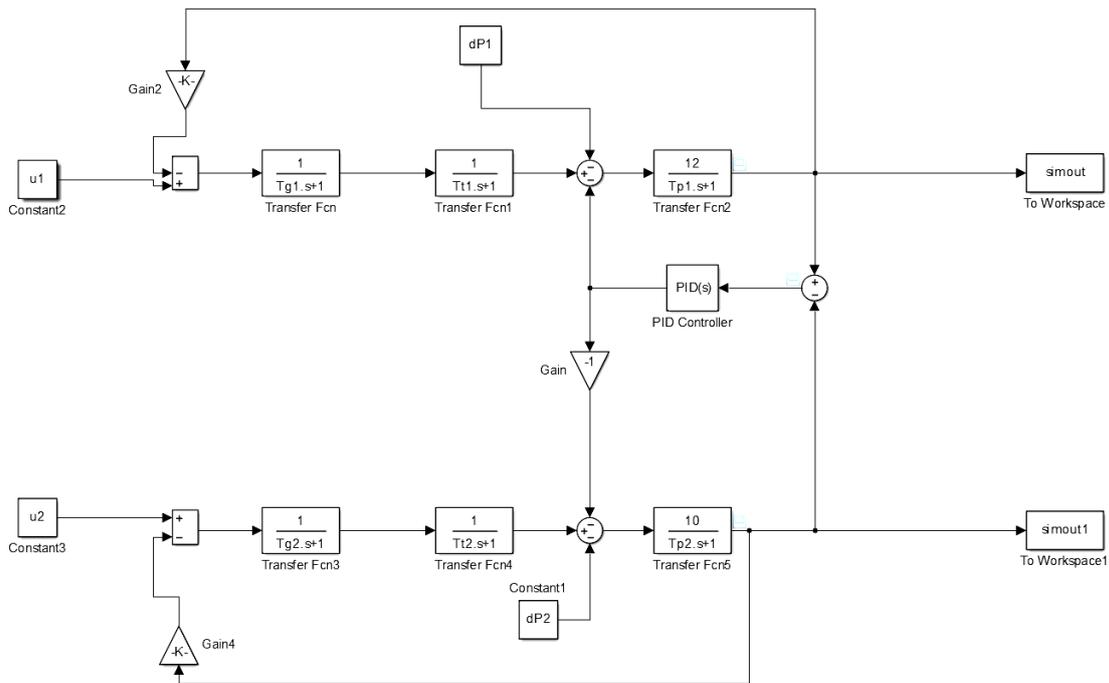
Figure 4. Two area power system with GA tuned PID controller
