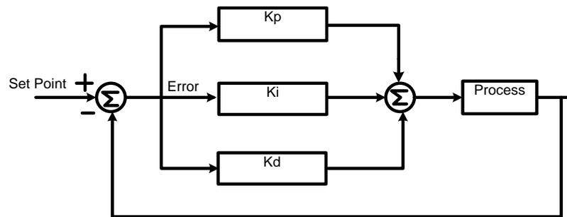
Figure 2. Block diagram of a PID Controller
