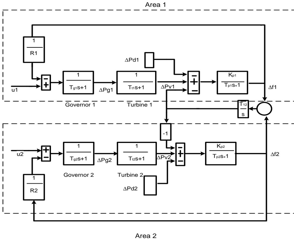
Figure 1. Block diagram of two area power system
