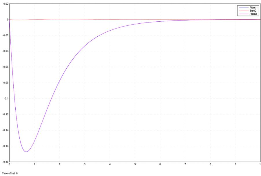
Figure 7. Deviation of frequency of two area power system with GA tuned PID controller
