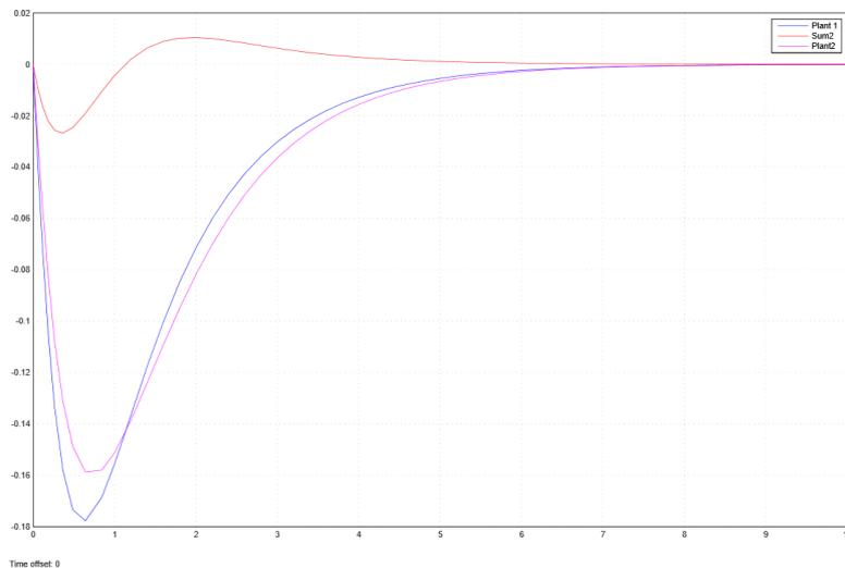
Figure 6. Deviation of frequency of two area power system without PID controller
