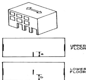
Fig. In-Plane Discontinuity in Vertical Elements Resisting Lateral Force
