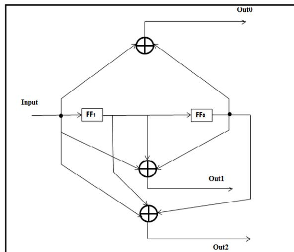
Figure1. Convolutional Encoder ( $K=3, k=1$  and  $n=3$ )
