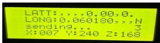
*Figure 10 : Output of GPS on LCD Screen*
