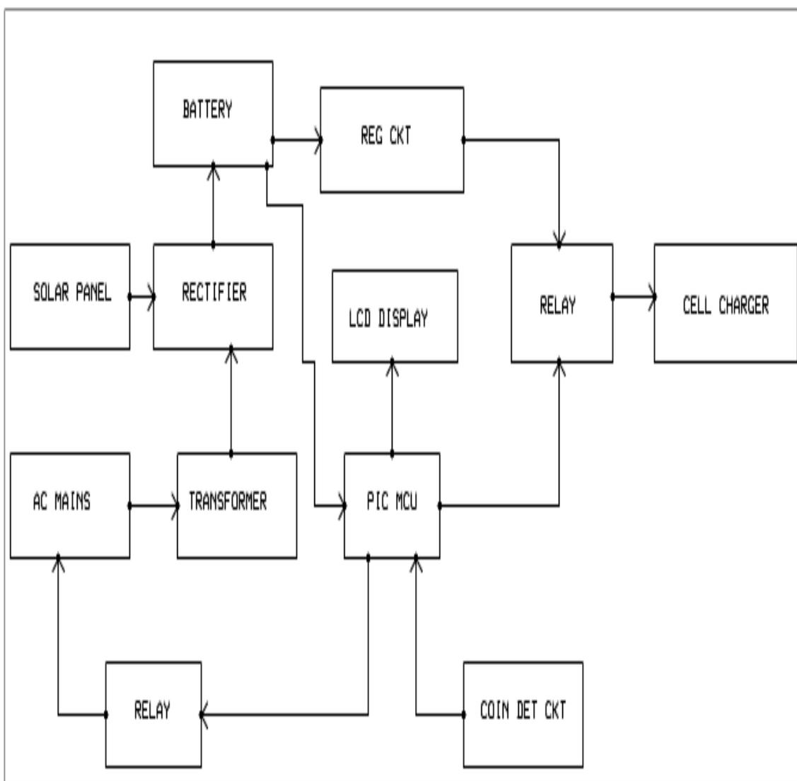
Figure 1. Block diagram of coin paid mobile charging system.
