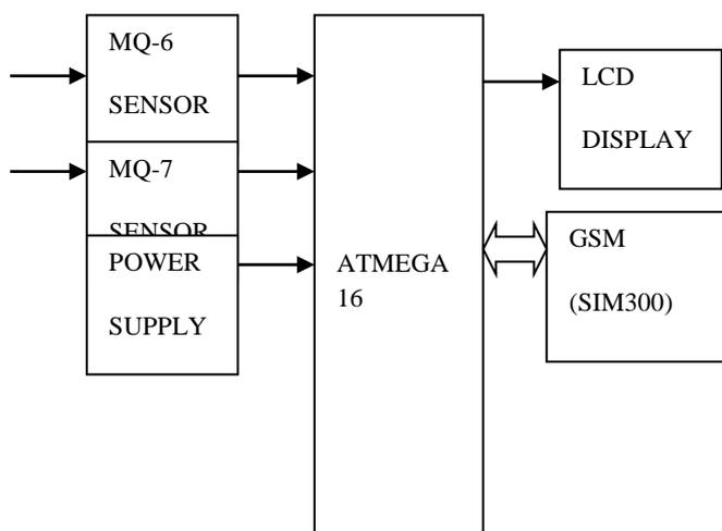
Fig. 1: Block schematic.[Ref3,4]
